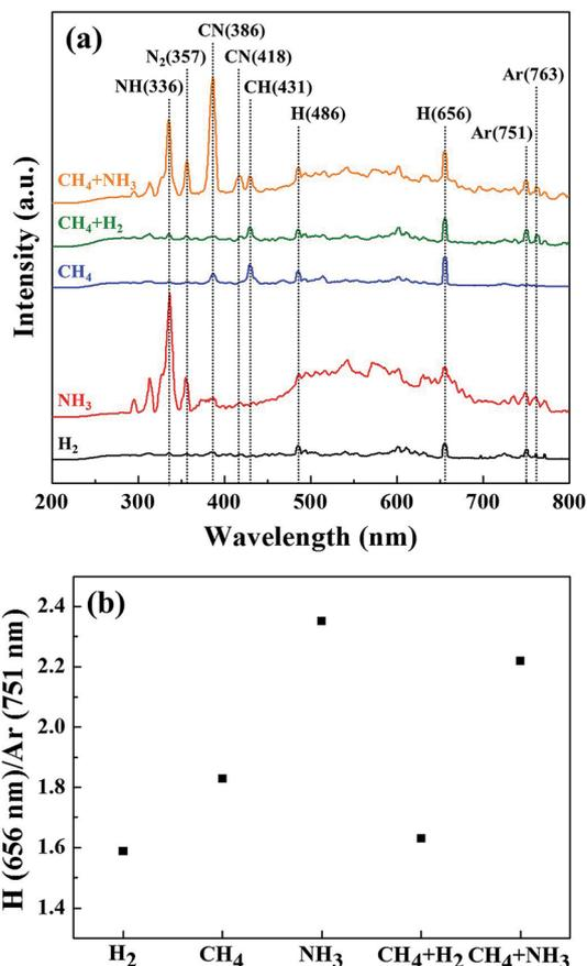
**Fig. 3** (a) OES spectra for H<sub>2</sub>, NH<sub>3</sub>, CH<sub>4</sub> + H<sub>2</sub> (1 : 1), and CH<sub>4</sub> + NH<sub>3</sub> (1 : 1). 5% Ar was added to the gases for the rough estimation of the hydrogen concentration in the plasma. (b) The peak intensity ratios of H (656 nm)/Ar (751 nm) for (a).
