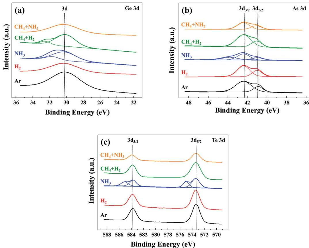
Fig. 6 XPS narrow scan data of (a) Ge 3d, (b) As 3d, and (c) Te 3d on the OTS material surfaces etched by Ar, H<sub>2</sub>, NH<sub>3</sub>, CH<sub>4</sub> + H<sub>2</sub> (1 : 1), and CH<sub>4</sub> + NH<sub>3</sub> (1 : 1) gases. The OTS material was etched ~20 nm.
