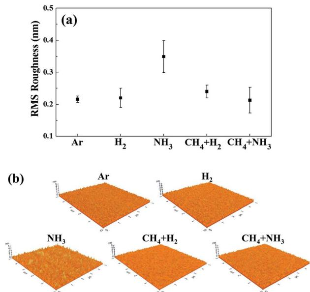
Fig. 4 (a) Surface roughness measured by AFM after the partial etching ( $\sim 20$  nm) of the 25 nm thick OTS material using Ar,  $H_2$ ,  $NH_3$ ,  $CH_4 + H_2$ , and  $CH_4 + NH_3$  gases. (b) AFM images of etched OTS materials in  $5 \mu m \times 5 \mu m$  area.
