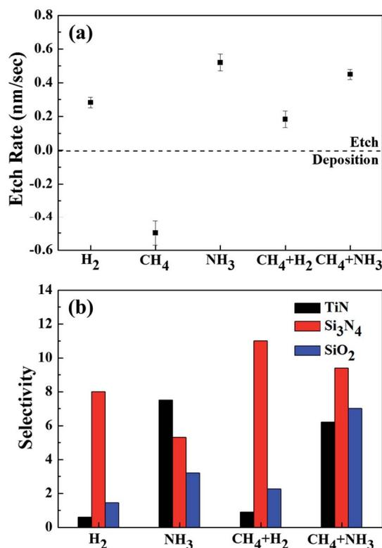
Fig. 2 (a) Etch rates of the OTS material using  $\text{H}_2$ ,  $\text{CH}_4$ ,  $\text{NH}_3$ ,  $\text{CH}_4 + \text{H}_2$  (1 : 1), and  $\text{CH}_4 + \text{NH}_3$  (1 : 1). (b) Etch selectivities of OTS over TiN,  $\text{Si}_3\text{N}_4$ , and  $\text{SiO}_2$  for the etch conditions in (a).
