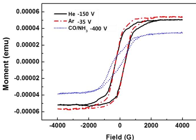
FIG. 8. Magnetization behaviors of patterned MTJs etched using He , Ar, and CO/NH<sub>3</sub>.
