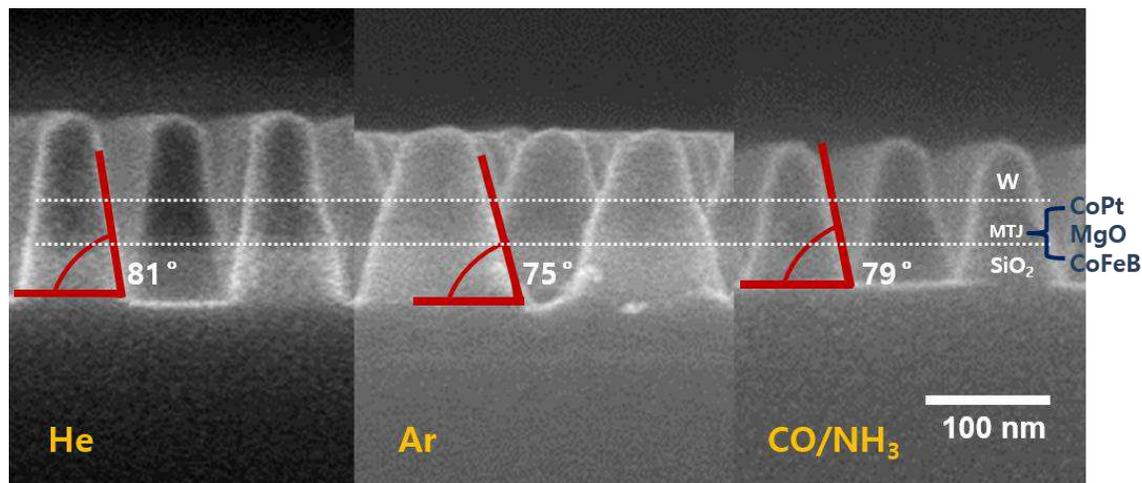
Figure 7. FE-SEM images of the etched MTJ patterns etched using the He, Ar and CO/NH<sub>3</sub> gases.
