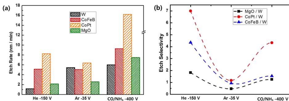
Figure 4. Etch rates of MTJ materials and W and etch selectivities of MTJ materials over W (a) etch rates of MTJ materials and (b) etch selectivities of MTJ materials over W.
