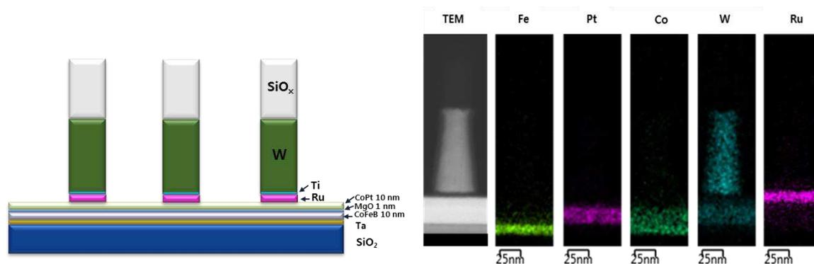
Figure 2. Schematic diagram of the MTJ stack and structure of the MTJs taken by transmission electron microscopy (TEM).
