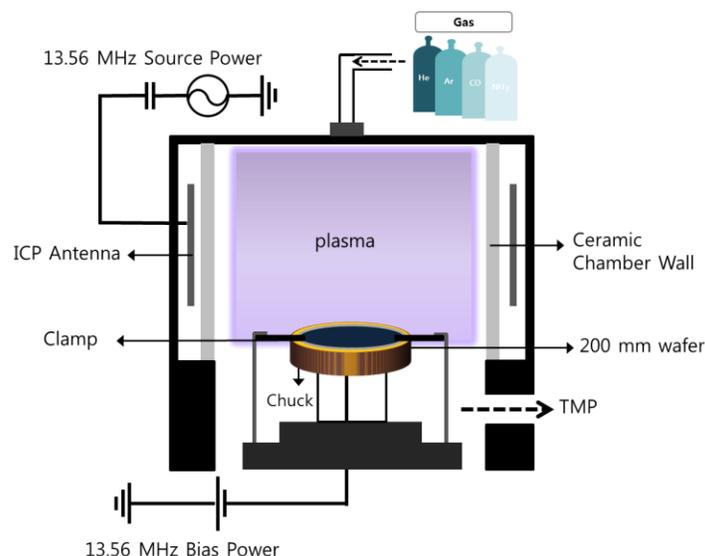
Figure 1. Schematic diagram of the ICP etcher used in this study.
