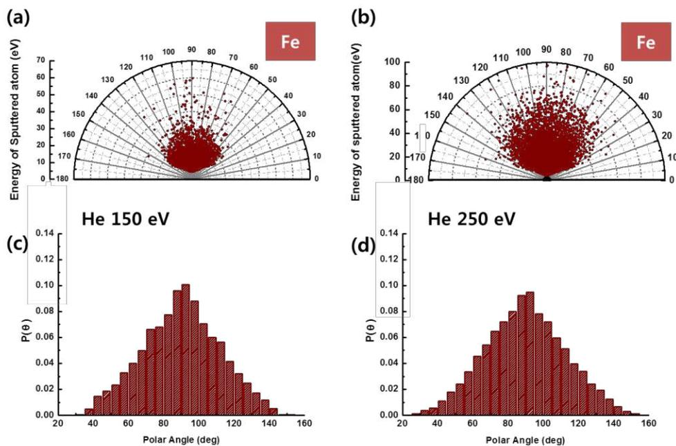
Figure 5. Energy and angular distribution of sputtered Fe in CoFeB with (a) 150 eV He ion and (b) 250 eV He ion by SRIM simulation. Angular distribution probability of sputtered Fe atom with (c) 150 eV He ion and (d) 250 eV He ion.
