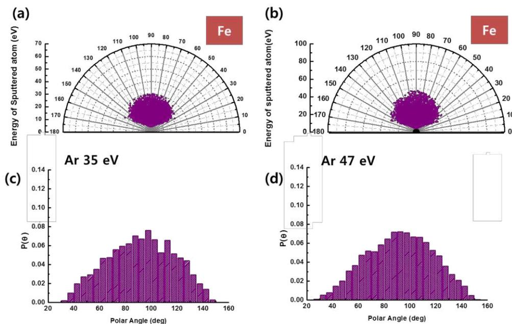
Figure 6. Energy and angular distribution of sputtered Fe in CoFeB with (a) 35 eV Ar ion and (b) 47 eV Ar ion by SRIM simulation. Angular distribution probability of sputtered Fe atom with (c) 35 eV Ar ion and (d) 47 eV Ar ion.
