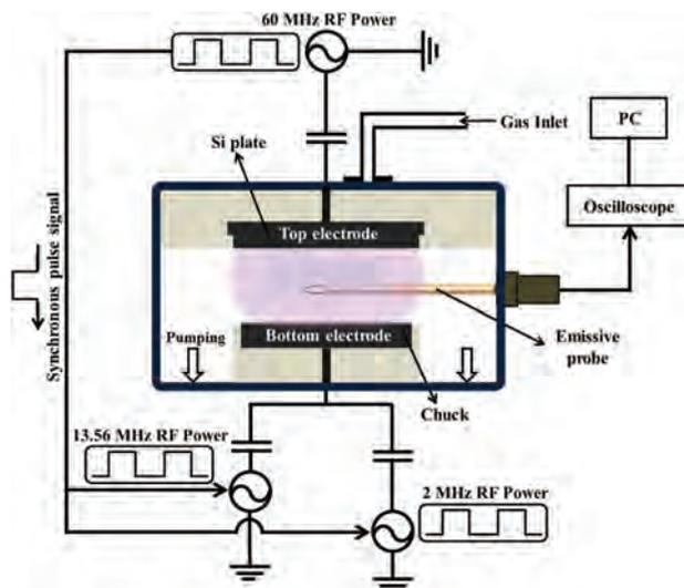
**Figure 1.** Schematic diagram of synchronized rf pulsing in the triple-frequency CCP. A pulsed 60 MHz source power was applied to the top electrode to control the plasma properties. Pulsed 13.56/2 MHz bias powers were applied to the bottom electrode to control both the plasma properties and ion energy at the substrate.
