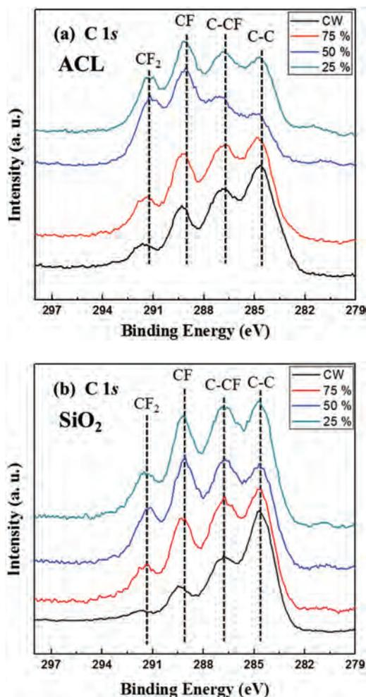
**Figure 9.** XPS narrow scan data of C 1s on the etched ACL and SiO<sub>2</sub> surface as a function of 13.56 MHz pulse duty percentages. SiO<sub>2</sub> samples were etched to 1.6 μm of etch depth in the 60/13.56/2 MHz triple-frequency CCP. The process conditions are the same as those in Figure 7.
