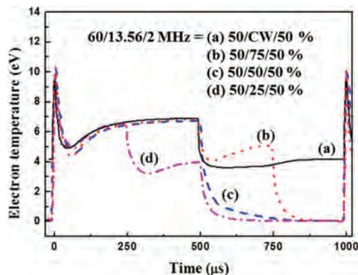
**Figure 6.** Instant electron temperature estimated as a function of 13.56 MHz pulse duty percentages in the synchronously pulsed plasmas. Ar gas at an operating pressure of 30 mTorr was used. The 13.56 MHz pulse duty percentage was varied from 100% (CW) to 25%, while maintaining the 60 MHz/13.56 MHz/2 MHz rf power = 200 W/200 W/900 W, respectively.
