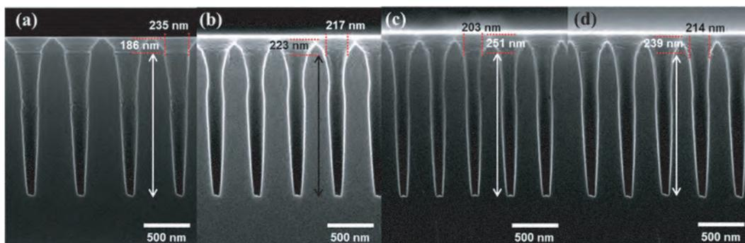
**Figure 8.** Etch profiles of ACL masked SiO<sub>2</sub> after etching as a function of 13.56 MHz pulse duty percentages in the pulsed triple-frequency CCP. The etch time of SiO<sub>2</sub> was varied to obtain an etch depth of about 1.6 μm. The process conditions are the same as those in Figures 7(a–d) for 100% (CW), 75%, 50%, and 25% of 13.56 MHz pulse duty percentage, respectively, while keeping the pulse duty percentages of 60 MHz and 2 MHz at 50%.
