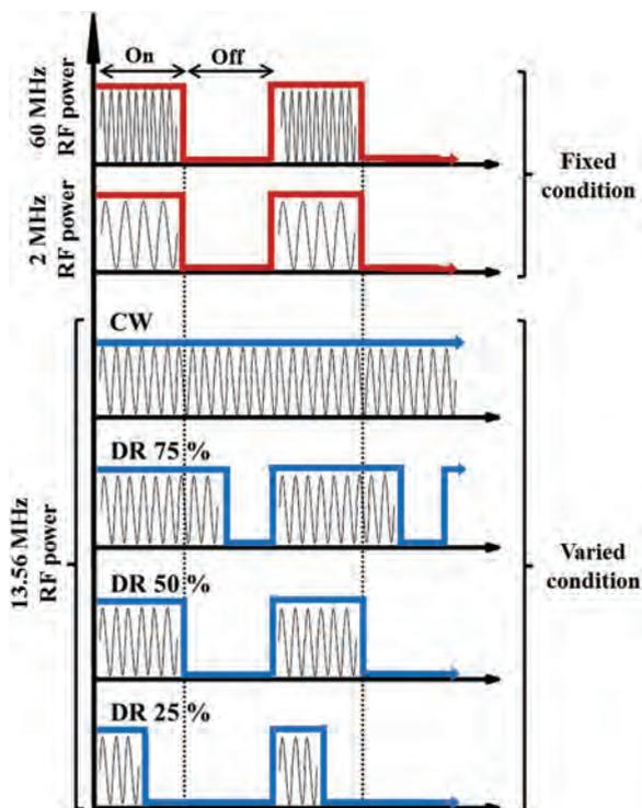
**Figure 5.** Schematic diagram of the pulse synchronization between the 60 MHz source pulsing and the 13.56/2 MHz bias pulsing for various 13.56 MHz pulse duty percentages in the synchronized triple-frequency CCP.
