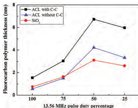
**Figure 10.** The steady-state thickness of the fluorocarbon polymer on the etched ACL and SiO<sub>2</sub> surface calculated from XPS C 1s narrow scan data shown in Figure 9.
