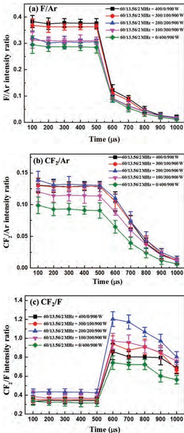
**Figure 3.** Time-resolved optical emission intensity ratios of (a) F/Ar, (b) CF<sub>2</sub>/Ar and (c) CF<sub>2</sub>/F as a function of 60/13.56 MHz rf power ratios using Ar/C<sub>4</sub>F<sub>6</sub>/O<sub>2</sub> gas mixtures in synchronously pulsed plasmas. The other conditions are the same as those in Figure 2.
