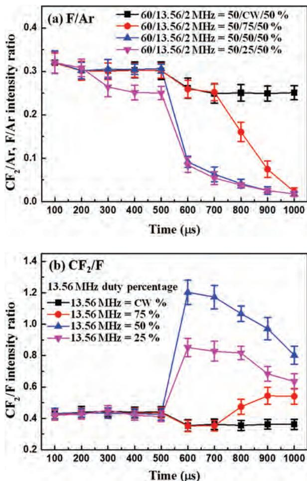
**Figure 7.** Time-resolved optical emission intensity ratios of (a) F/Ar and (b) CF<sub>2</sub>/F as a function of 13.56 MHz pulse duty percentages using Ar/C<sub>4</sub>F<sub>6</sub>/O<sub>2</sub> gas mixtures in the synchronously pulsed plasmas. The other conditions are the same as those in Figure 6.
