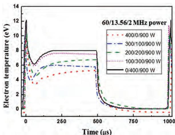
**Figure 2.** Instant electron temperature estimated as a function of the 60/13.56 MHz rf power ratios in the synchronously pulsed plasmas. Ar gas at an operating pressure of 30 mTorr was used. The pulse duty ratio and the pulse frequency were kept at 50% and 1 kHz, respectively. 60/13.56/2 MHz rf powers were varied as 400/0/900 W, 300/100/900 W, 200/200/900 W, 100/300/900 W, and 0/400/900 W, respectively.
