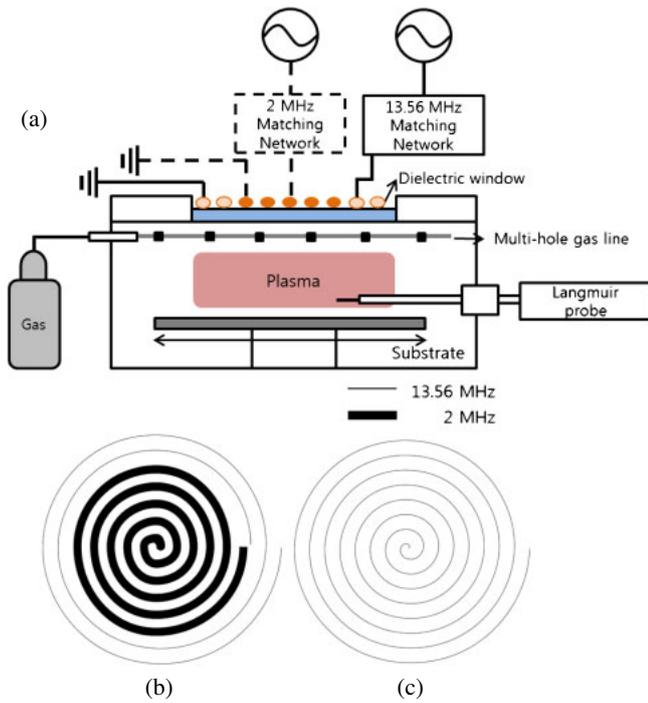
**Fig. 1.** (Color online) (a) Schematic diagram of ICP system used in this experiment. (b) Dual-frequency ICP source shape using frequency of 13.56 and 2 MHz. (c) Single-frequency ICP source shape using frequency of 13.56 MHz.
