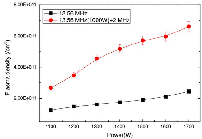
**Fig. 2.** (Color online) Plasma density of dual-frequency ICP source and single-frequency ICP source as a function of total power. For the dual-frequency mode, the 13.56 MHz rf power was kept at 1000 W and the 2 MHz rf power was varied from 100 to 800 W with 10 mTorr Ar.
