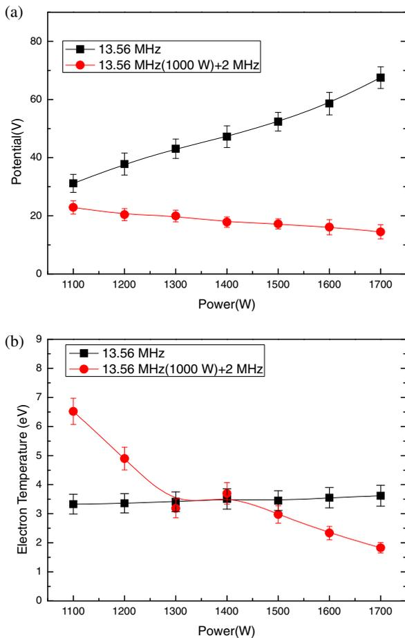
**Fig. 3.** (Color online) (a) Plasma potential and (b) electron temperature of dual-frequency ICP source and single-frequency ICP source with 10 mTorr Ar.
