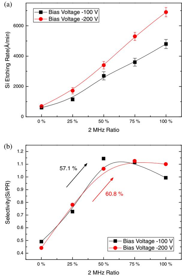
**Fig. 5.** (Color online) (a) Silicon etching rate and (b) etching selectivity of silicon over photoresist measured as a function of ratio of 13.56 and 2 MHz rf powers while maintaining the total rf power at 1000 W. The rf frequency for substrate biasing was 12.56 MHz (−100 and −200 V) and a 20 mTorr CF<sub>4</sub>/Ar (10 : 1) gas mixture was used.
