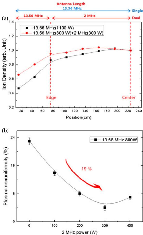
**Fig. 4.** (Color online) (a) Ion density measured with a Langmuir probe along the chamber centerline for the single-frequency source power (13.56 MHz, 1100 W) and the dual-frequency source power (13.56 MHz, 800 W and 2 MHz 300 W) with 10 mTorr Ar. (b) Plasma nonuniformity of the dual-frequency ICP source measured with the Langmuir probe as a function of 2 MHz rf power from 0 to 400 W in addition to 800 W at rf power 13.56 MHz.
