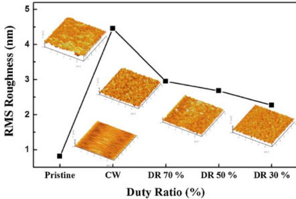
**Fig. 6.** (Color online) AFM surface roughness of the etched CoFeB as a function of pulse duty percentage using a CO/NH<sub>3</sub> gas combination in the ICP system. The etch conditions are the same as those in Fig. 4.
