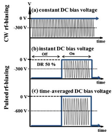
Fig. 2. (Color online) (a) CW RF biasing at –300 V of constant DC bias voltage condition. (b) and (c) show the rf pulsed biasing with the 50% duty ratio at –300 V of DC bias voltage condition for instant DC biasing and time-averaged DC biasing, respectively.
