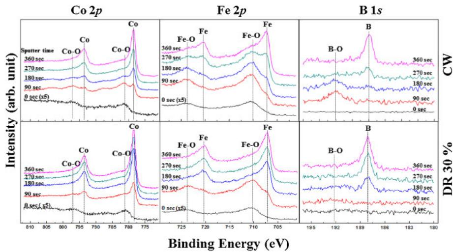
**Fig. 4.** (Color online) XPS narrow scan data of Co 2p, Fe 2p, and B 1s during the depth profiling of the CoFeB surface etched with CW and 30% pulse duty percentage. The samples were etched for 3 min with the time-averaged DC bias voltage condition of  $-300$  V and the other etch conditions are the same as those in Fig. 3.
