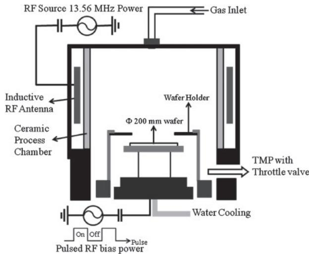
Fig. 1. Schematic diagram of the ICP etching system used in this study.
