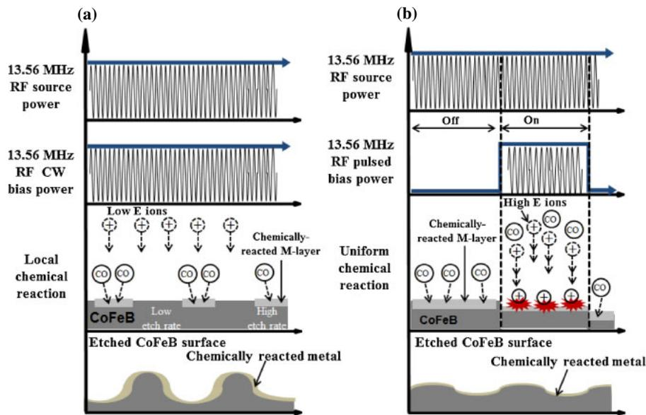
**Fig. 7.** (Color online) Schematic drawing of one of the possible reaction mechanisms during the etching using CW biasing (100% pulse duty cycle) and 50% pulsed duty cycle.
