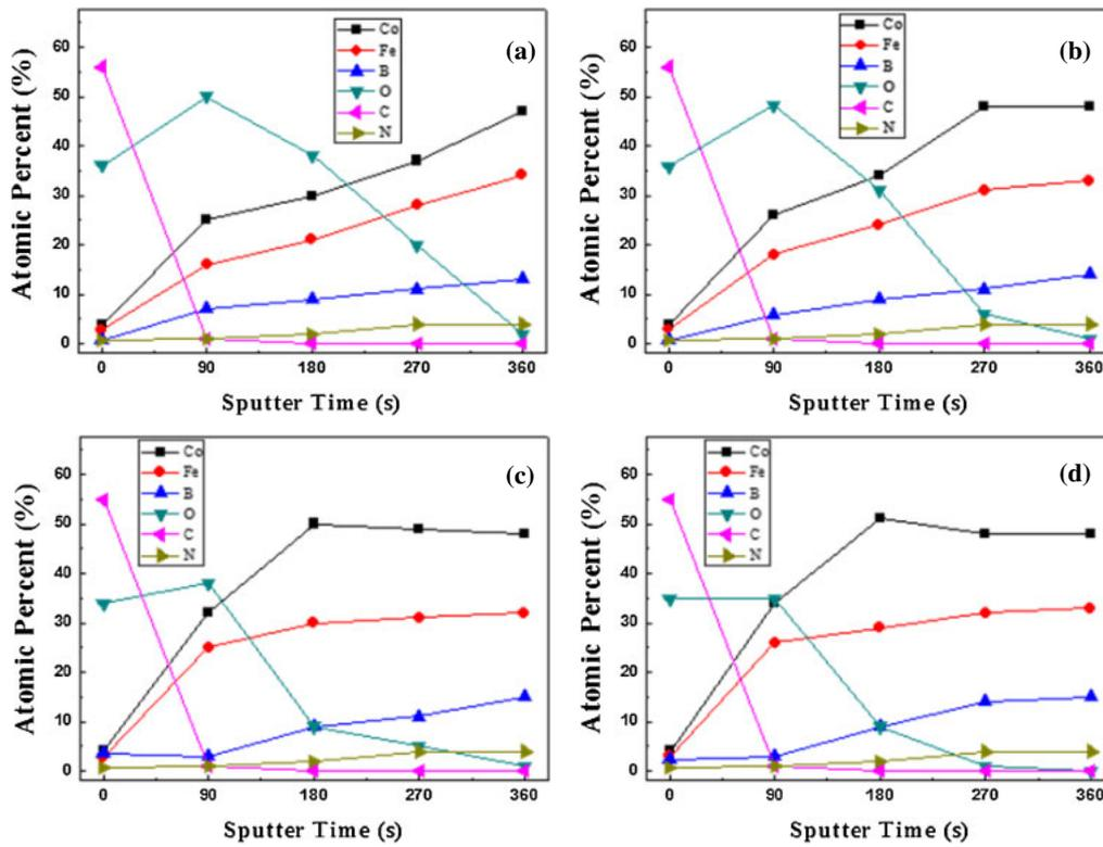
**Fig. 5.** (Color online) Relative atomic percentages of the etched CoFeB surface measured by XPS depth profiling as a function of Ar<sup>+</sup> ion sputter etch time for the CoFeB samples etched for various pulse duty percentages including the CoFeB etched with the CW biasing. (a) CW, (b) DR 70%, (c) DR 50%, and (d) DR 30%. The etch conditions are the same as those in Fig. 4.
