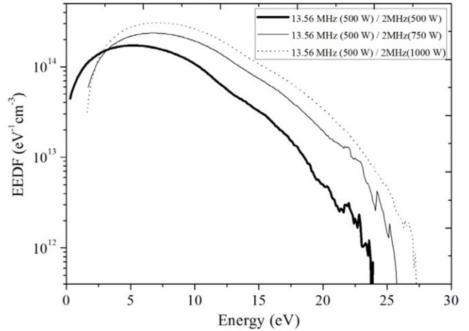
**Figure 2.** Evolution of electron energy distribution functions with low-frequency power ( $P_{2\text{MHz}}$ ) at a pressure of 10 mTorr, in a discharge of Ar(400 sccm)/CF<sub>4</sub>(100 sccm). The high-frequency ( $P_{13.56\text{MHz}}$ ) power is kept constant at 500 W.
