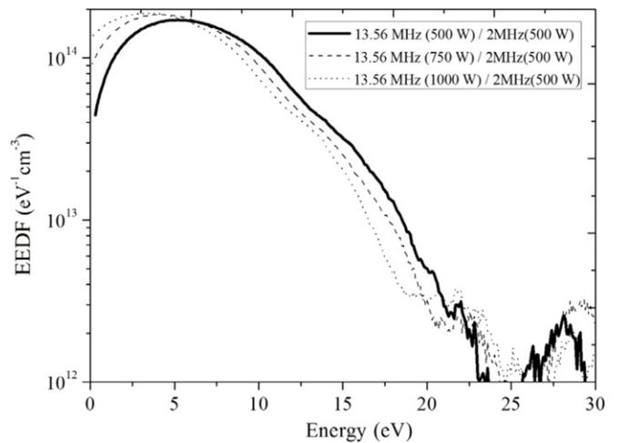
**Figure 3.** Evolution of electron energy distribution functions with high-frequency power ( $P_{13.56\text{MHz}}$ ) at a pressure of 10 mTorr, in a discharge of Ar(400 sccm)/CF<sub>4</sub>(100 sccm). The low-frequency power ( $P_{2\text{MHz}}$ ) is kept constant at 500 W.
