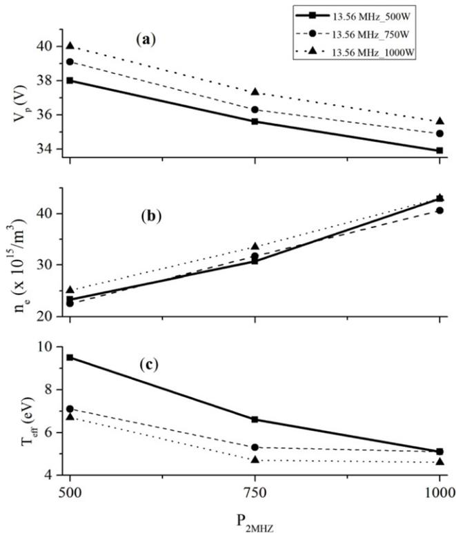
**Figure 5.** Effect of  $P_{2\text{MHz}}$  (a) plasma potential (b) plasma density and (c) effective electron temperature at the three chosen values of RF power (500, 750 and 1000 W) of both RF frequency powers.
