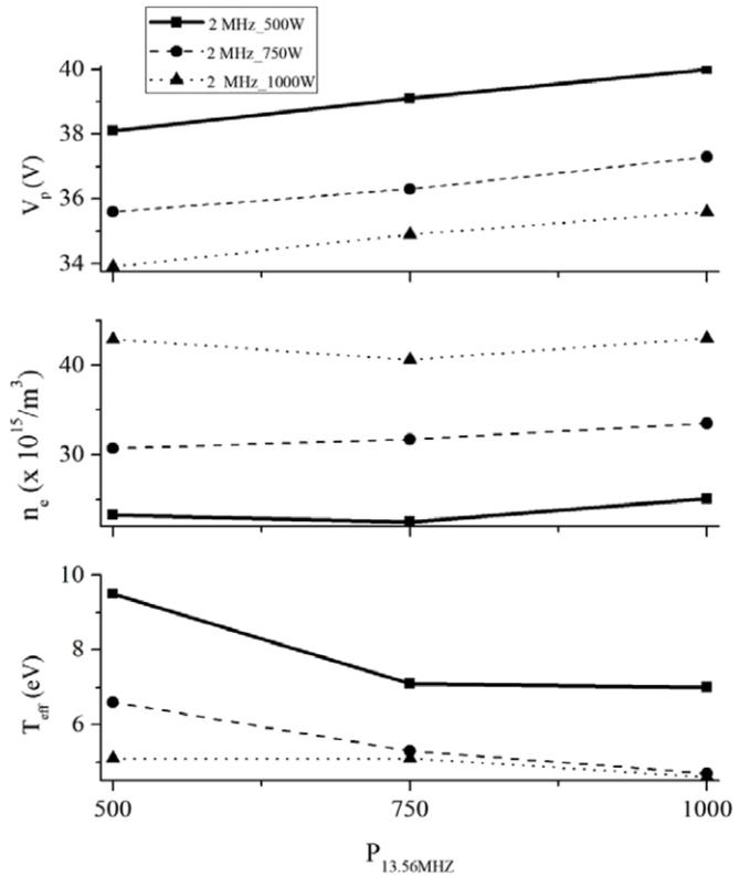
**Figure 6.** Effect of  $P_{13.56\text{MHz}}$  (a) plasma potential (b) plasma density and (c) effective electron temperature at the three chosen values of RF power (500, 750 and 1000 W) of both RF frequency powers.
