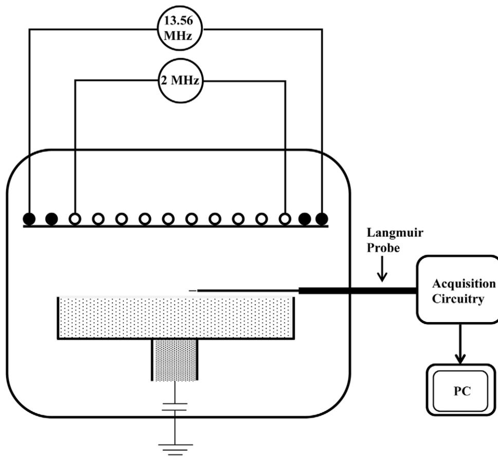
**Figure 1.** Schematic diagram (not to scale) of the discharge chamber and Langmuir probe system used in this study.
