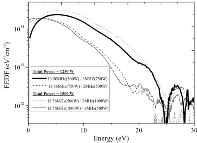
**Figure 4.** Evolution of electron energy distribution functions at a fixed total power of (a) 1250 W and (b) 1500 W while varying the RF power ratios of 2 and 13.56 MHz.
