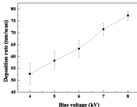
**Figure 2.** Effect of ac-bias voltage (4–8 kV, 20 kHz ac power) to the substrate on the deposition rate of  $\text{SiO}_x$  thin film. HMDS (400 sccm)/ $\text{O}_2$  (20 slm)/He (5 slm)/Ar (3 slm) was flowed to the remote-type modified DBD source operated at 7 kV, 30 kHz.
