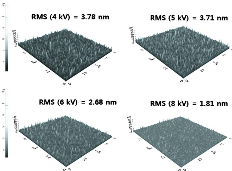
**Figure 8.** (Color online) Surface roughness of  $\text{SiO}_x$  film deposited by AFM as a function of ac-bias voltage. The deposition conditions are the same as those shown in Fig. 2.
