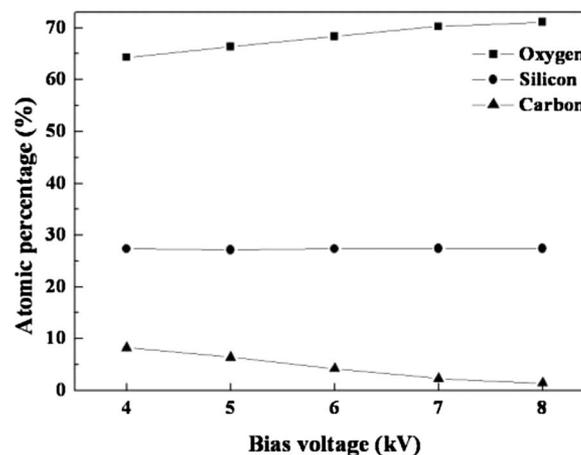
**Figure 3.** Atomic percentage of the deposited  $\text{SiO}_x$  thin film investigated by XPS as a function of ac-bias voltage from 4 to 8 kV. The other deposition conditions are the same as those in Fig. 2.
