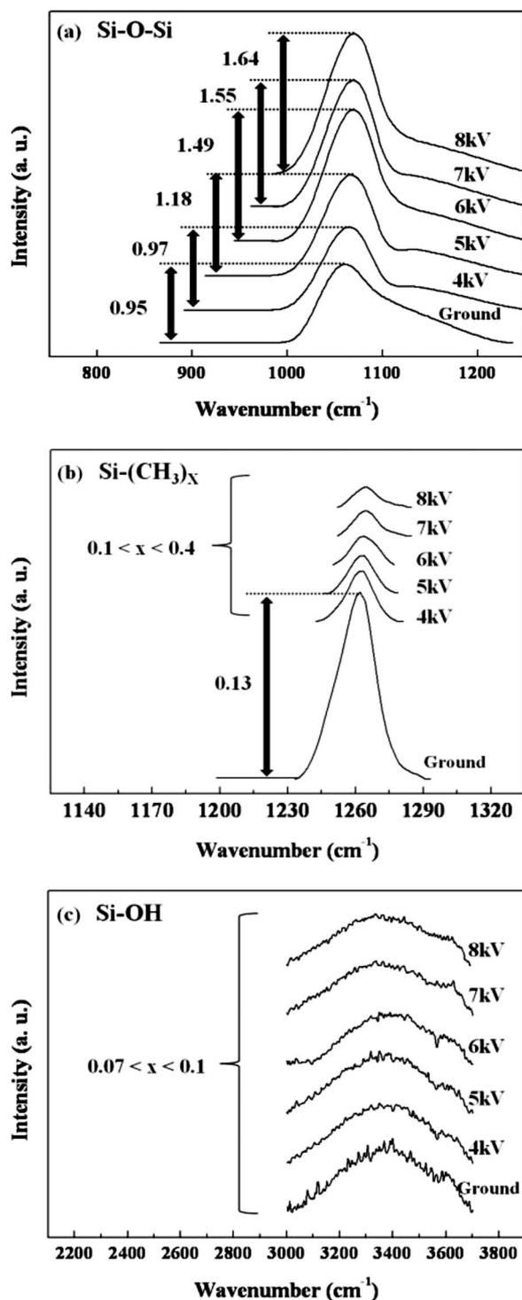
**Figure 4.** FTIR spectra of the  $\text{SiO}_x$  thin films deposited at various ac-bias voltages. Thickness of the deposited  $\text{SiO}_x$  thin film was kept at 200 nm. The other deposition conditions are the same as those shown in Fig. 2. (a) for Si-O-Si bonding, (b) for Si-( $\text{CH}_3$ ) $_x$  bonding, and (c) for Si-OH bonding.
