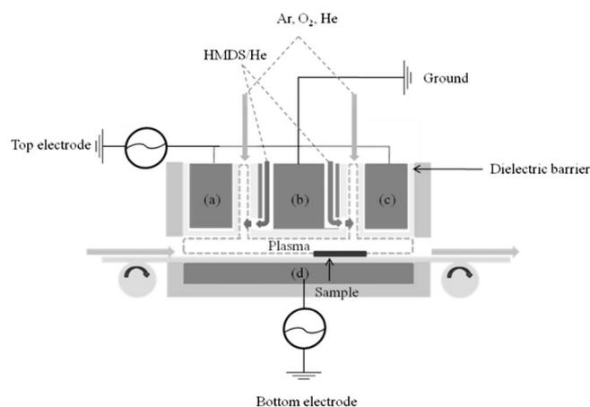
**Figure 1.** Schematic diagram of the AP-PECVD inline system with a remote-type modified DBD source and ac-biased substrate used to deposit the  $\text{SiO}_x$  films.
