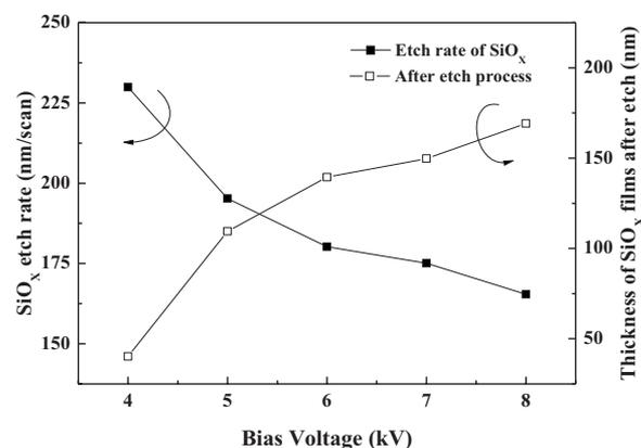
**Figure 6.** Etch rate of the  $\text{SiO}_x$  deposited as a function of ac-bias voltage in atmospheric pressure etching equipment in  $\text{N}_2$  (40 slm)/He (1 slm)/ $\text{NF}_3$  (500 sccm) and using 2 kW of 40 kHz pulse power. The  $\text{SiO}_x$  deposition conditions are the same as those shown in Fig. 2.
