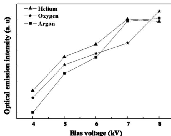
**Figure 5.** Relative optical emission intensities measured as a function of ac-bias voltage. The operating conditions are the same as those shown in Fig. 2.
