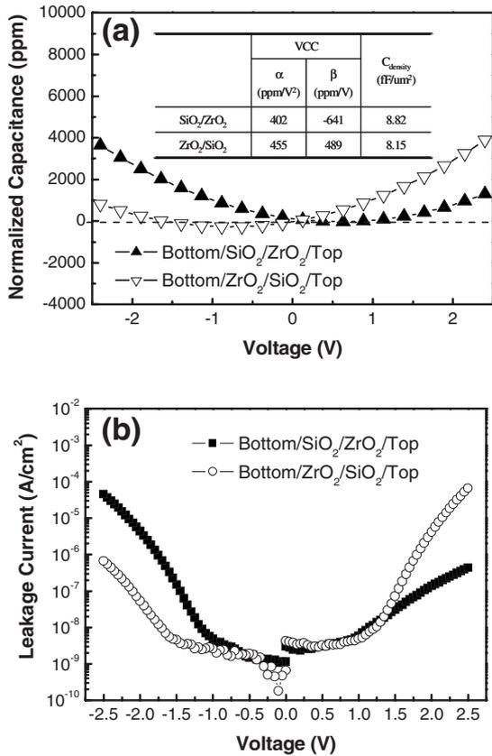
FIG. 2. (a) Normalized capacitance characteristics for a MIM capacitor with ZrO<sub>2</sub>/SiO<sub>2</sub> bilayer stack and (b)  $I$ - $V$  characteristics of such a structure. The inset shows VCC  $\alpha$  and  $\beta$  and capacitance density ( $C_{\text{density}}$ ) as a function of the dielectric stack sequence.
