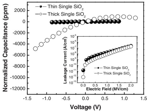
FIG. 4. Normalized capacitance of MIM capacitors with a single-layer  $\text{SiO}_2$  dielectric as a function of  $\text{SiO}_2$  thickness. The inset shows the leakage current of the MIM capacitor as a function of applied electric field. The capacitances of the thin  $\text{SiO}_2$  and thick  $\text{SiO}_2$  MIM capacitors are measured from  $-0.8$  to  $0.8$  V, and from  $-1.2$  to  $1.2$  V, respectively.
