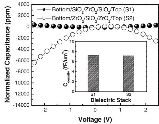
FIG. 3. Normalized capacitance of MIM capacitors with SiO<sub>2</sub>/ZrO<sub>2</sub>/SiO<sub>2</sub> and ZrO<sub>2</sub>/SiO<sub>2</sub>/ZrO<sub>2</sub> stacks. Both stacks, denoted as S1 and S2, respectively, have similar capacitance density, as the inset shows, but significantly different quadratic VCC values depending on the dielectric deposition sequence.
