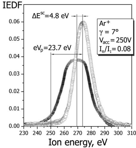
FIG. 2. Normalized IEDFs for the primary (white symbols) and reflected (dark symbols) ion beams.
