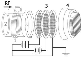
FIG. 1. Experimental setup for the low-angle forward-reflected neutral beam source. 1 rf antenna, 2 quartz chamber, 3 electrostatic electrodes, 4 reflector.
