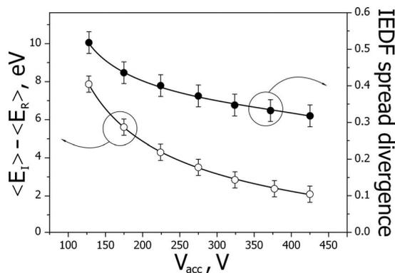
FIG. 3. Mean energy difference of the primary and reflected ion beams, and the energy distribution spread divergence as a function of the beam energy.
