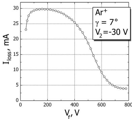
FIG. 6. Loss current at the second electrode as a function of the focusing potential.
