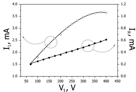
FIG. 8. Primary and reflected ion beam currents as a function of the acceleration potential at  $V_f=V_1 - V_2=\text{const}$ .
