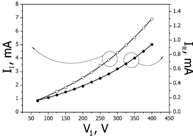
FIG. 9. Primary and reflected ion beam currents as a function of the acceleration potential at  $V_2 = \text{const}$ .
