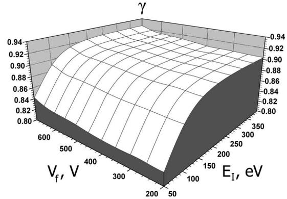
FIG. 11. Neutralization efficiency of the Ar beam as a function of the beam energy and focusing potential.
