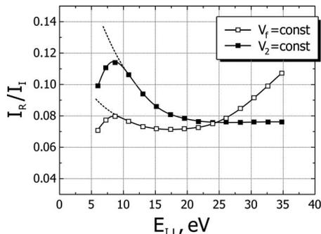
FIG. 10. Ratio of the reflected ion current and the primary ion current for two normalization methods. The dashed lines represent these dependences in the absence of the plasma potential influence on the ion current.
