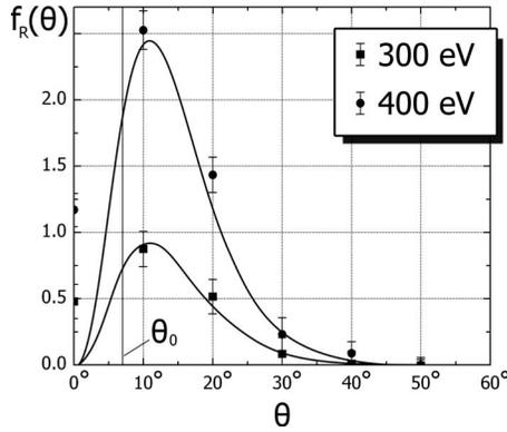
FIG. 5. Angular distribution of the neutral beam obtained from the beam etching rate measurements and the corresponding results of the angular distribution modeling for 300 and 400 eV beams.
