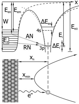
FIG. 4. Schematic diagram of AN, and RN and de-excitation during Ar<sup>+</sup> interaction with the reflector. The dashed lines at the top represent the undisturbed surface potential and atom energy levels.
