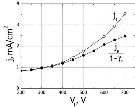
FIG. 7. Primary and reflected ion beam current growth as a function of the focusing potential.
