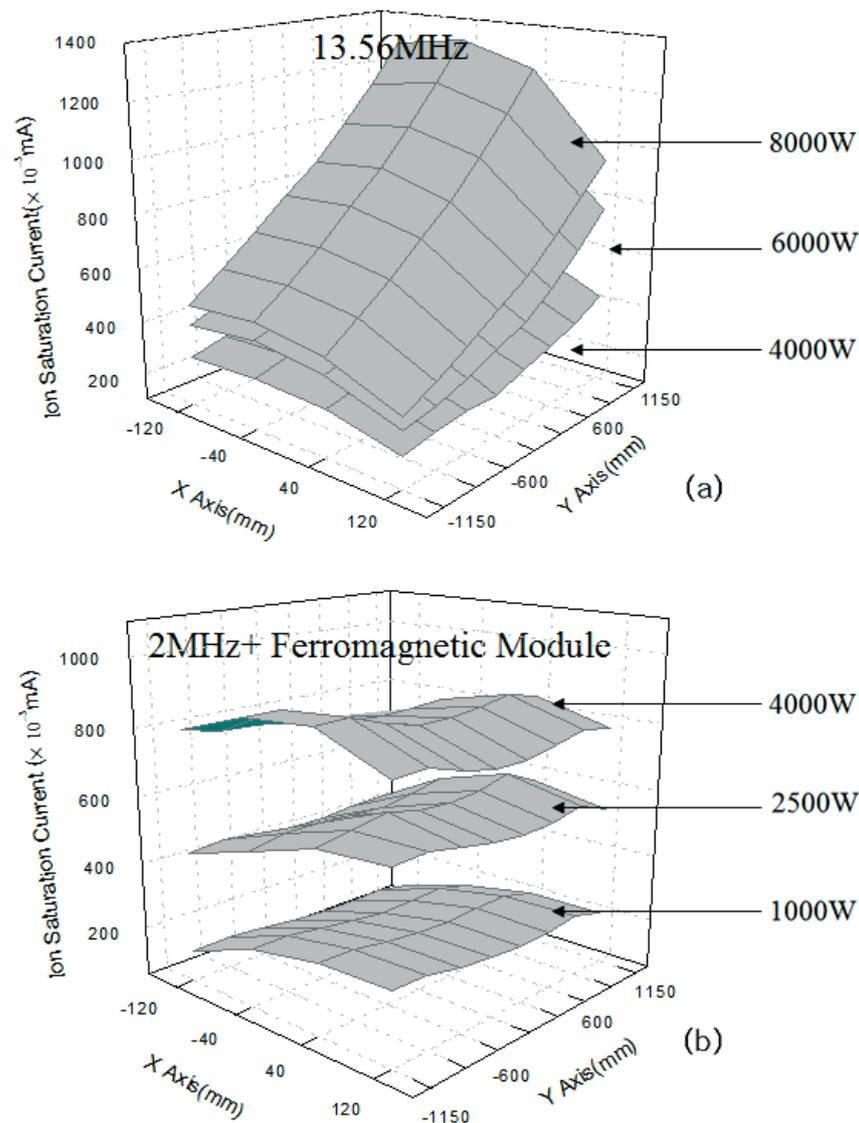
**Figure 4.** Plasma uniformity of (a) the 13.56 MHz source for an rf power of 4000–8000 W and of (b) the 2 MHz source with the ferromagnetic module for an rf power of 1000–4000 W measured using a movable electrostatic probe system biased at  $-65$  V at 20 mTorr Ar.
