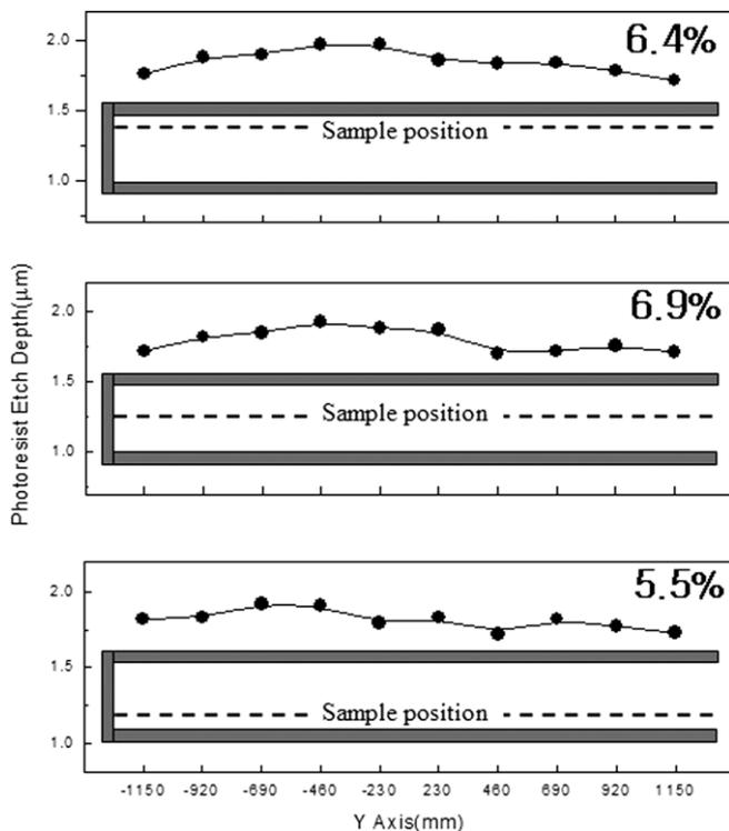
**Figure 5.** Photoresist etch uniformity measured at various antenna locations using the line-shaped ICP source operated at 2 MHz with a ferromagnetic module and at an rf power of 3500 W with 40 mTorr Ar/O<sub>2</sub> (7 : 3).
