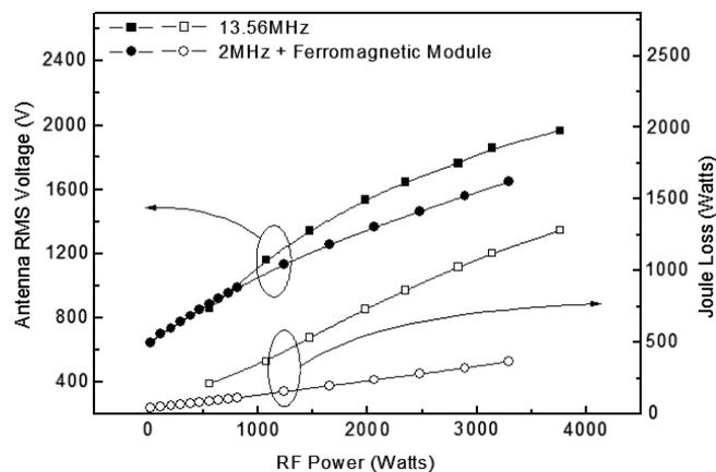
**Figure 3.** Rf rms voltage and Joule loss measured by an impedance analyzer on the antenna located close to the rf power input as a function of rf power with the ICP source operated at 13.56 and 2 MHz (with the ferromagnetic module) and at 20 mTorr Ar.
