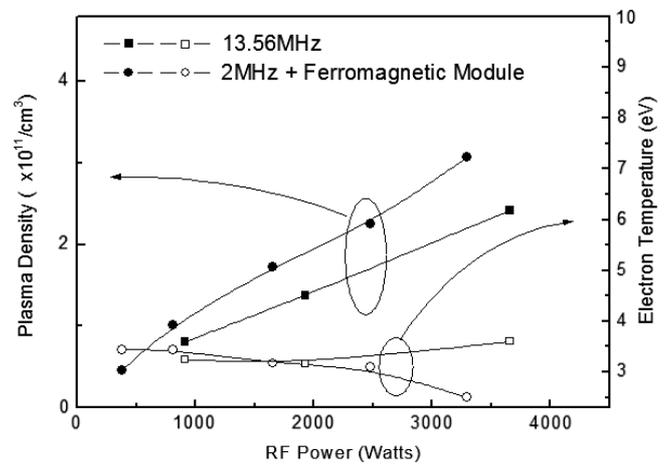
**Figure 2.** Plasma density and electron temperature measured by a Langmuir probe at 20 mTorr Ar as a function of rf power with the ICP source operated at 13.56 MHz and 2 MHz (with the ferromagnetic module).
