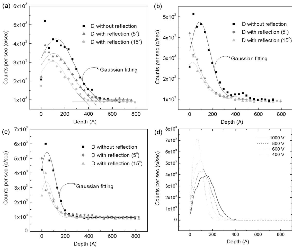
Fig. 2. SIMS depth profiles of deuterium ions or atoms on the silicon surface for various reflector angles for an incident ion energy of (a) 1 kV, (b) 600 V and (c) 400 V. (acceleration voltage: 400 V, 600 V and 1 kV; rf power: 300 W;  $D_2$  gas flow rate 15 sccm; implantation time: 30 min). (d) is the simulation result of the  $D^+$  implantation depth for various acceleration voltages.
