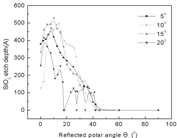
Fig. 4. SiO<sub>2</sub> etch depth distribution measured as a function of polar angle from the point of ion-beam reflection to measure the distribution of the reflected particles for incident angles from 5 to 20° (rf power: 400 W; SF<sub>6</sub> gas flow rate: 15 sccm; acceleration voltage: 400 V; etch time: 1 hour).
