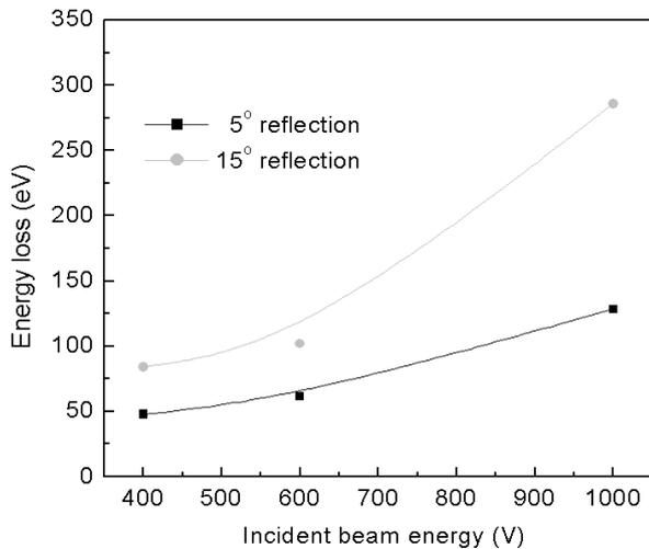
Fig. 3. Energy loss during reflection (neutralization) as a function of incident deuterium ion's energy from 400 V to 1 kV for incident angles of 5 and 15°.
