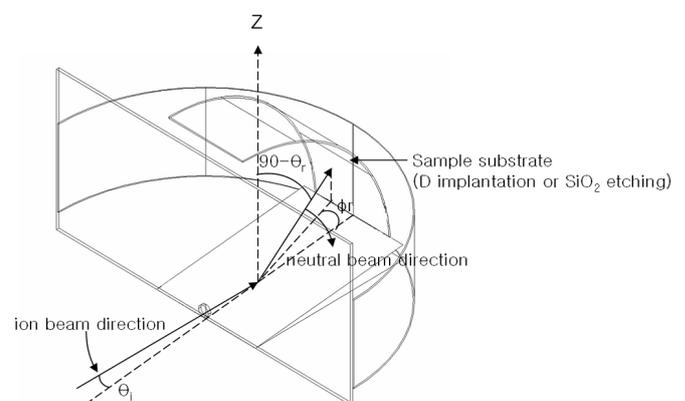
Fig. 1. Schematic diagram of the experimental system for the ion-beam reflection study.
