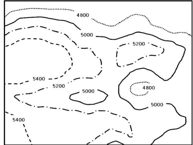
Fig. 4. Etch uniformity of PR on glass on the substrate area of 880 mm×660 mm measured at 5000 W of RF power, –100 V of dc bias voltage, and 15 mTorr of O<sub>2</sub> for the ICP source with the multiple U-type antenna.
