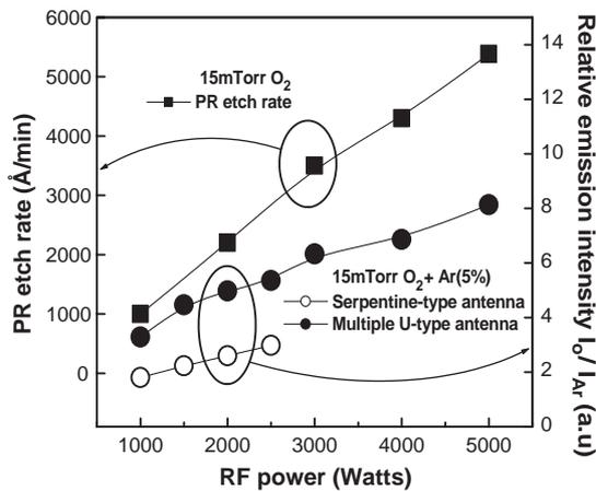
Fig. 3. Relative oxygen atomic density estimated by Ar actinometry for the serpentine-type antenna and the multiple U-type antenna and PR etch rate for the multiple U-type antenna as a function of RF power from 1000 to 5000 W at 15 mTorr O<sub>2</sub>. For the PR etching, –100 V of dc bias voltage was applied to the substrate. The substrate temperature was maintained at room temperature.
