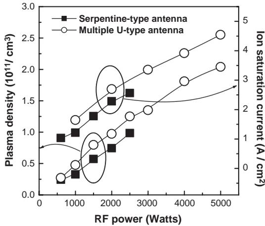
Fig. 2. Plasma density of 15 mTorr Ar and ion saturation current of 15 mTorr O<sub>2</sub> measured by a Langmuir probe at 7.5 m below the antenna and the center of the chamber as a function of RF power from 600 to 5000 W.
