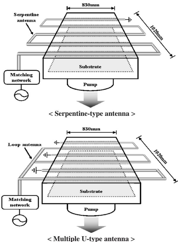
Fig. 1. Schematic diagrams of the serpentine-type antenna and the multiple U-type antenna as the internal ICP sources installed in the 1020 mm×830 mm rectangular chamber for the application to TFT–LCD processing.
