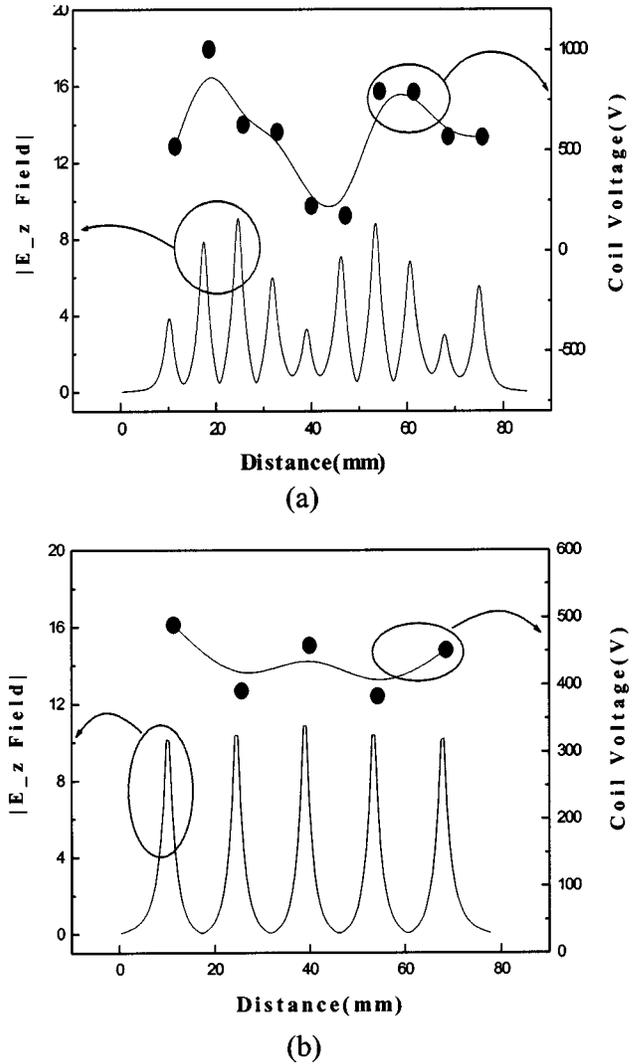
FIG. 2. Antenna voltages measured along the antenna line using a high voltage probe and the  $E_z$  field at each antenna position simulated by a F2L code for 2000 W and 15 mTorr Ar. (a) Serpentine-type antenna and (b) double-comb-type antenna.
