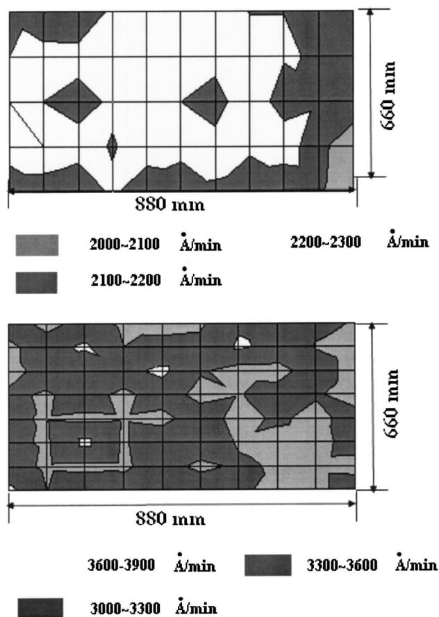
FIG. 4. (a) Etch uniformity of  $\text{SiO}_2$  measured at 5000 W of inductive power,  $-35$  V of dc bias voltage, and 15 mTorr of  $\text{SF}_6$  for a substrate area of  $880 \text{ mm} \times 660 \text{ mm}$ . (b) Etch uniformity of photoresist measured at 5000 W of rf power,  $-60$  V of dc bias voltage, and 15 mTorr of  $\text{O}_2$  for a substrate area of  $880 \text{ mm} \times 660 \text{ mm}$ .
