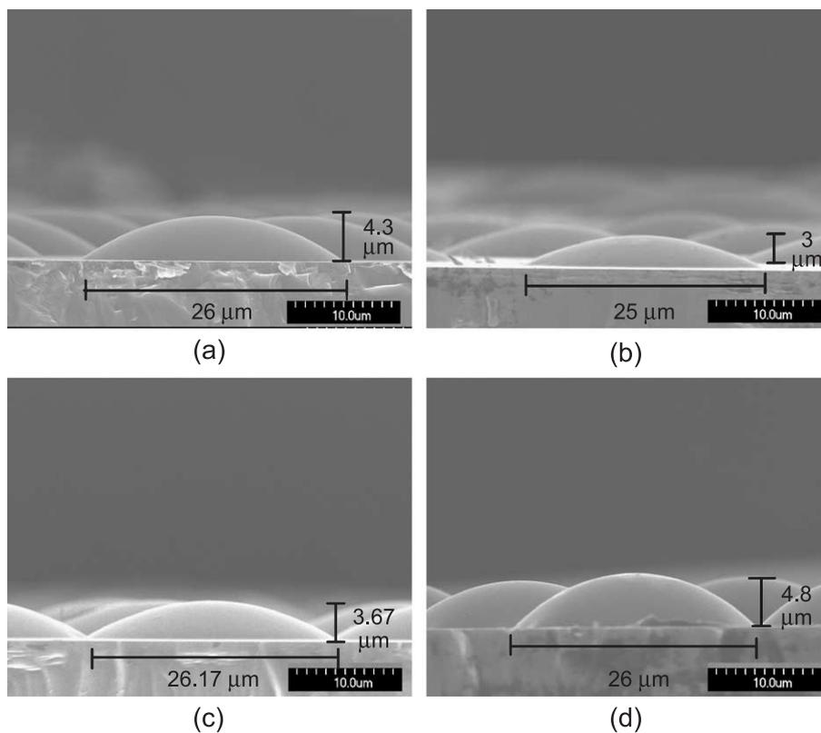
Fig. 4. SEM micrographs of the etched SiC micro-lens structures. (a) reflowed PR micro-lens, (b) HBr 0 sccm, (c) HBr 50 sccm, and (d) HBr 60 sccm (inductive power: 1400 W; bias voltage:  $-150$  V; HCl: 50 sccm; working pressure: 10 mTorr).
