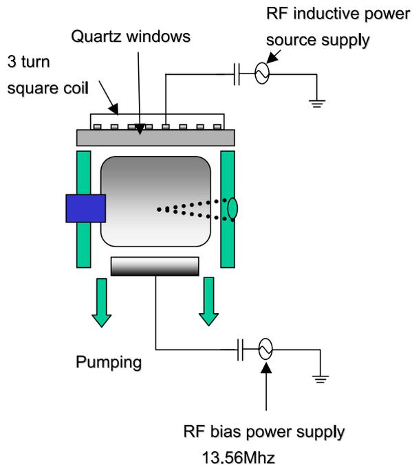
Fig. 1. Schematic diagram of the inductively coupled plasma etch system used in this study.
