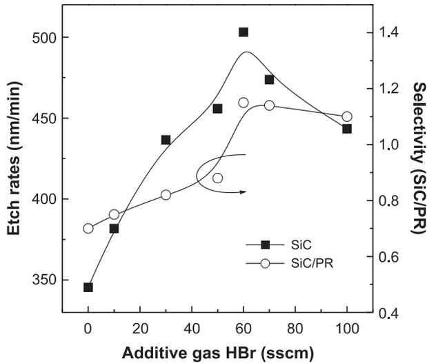
Fig. 3. Measured SiC etch rates and PR selectivity as a function of additive HBr (inductive power: 1400 W; bias voltage:  $-150$  V; HCl: 50 sccm; working pressure: 10 mTorr).
