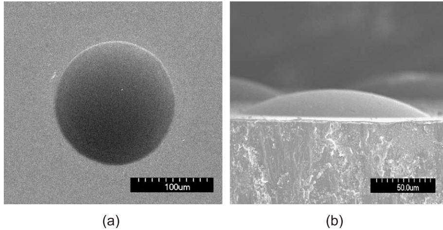
Fig. 5. SEM micrographs of the etched SiC micro-lens having about 200- $\mu\text{m}$  diameter (inductive power: 1400 W; bias voltage:  $-150$  V; gas composition: HCl 50 sccm+HBr 60 sccm; working pressure: 10 mTorr).
