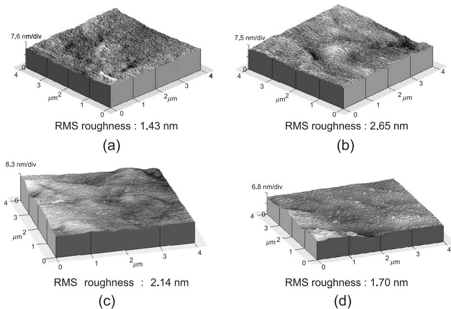
Fig. 6. AFM micrographs of the etched SiC surfaces. (a) SiC before etching, (b) HBr 0 sccm, (c) HBr 50 sccm, and (d) HBr 60 sccm (inductive power: 1400 W; bias voltage:  $-150$  V; HCl 50 sccm; working pressure: 10 mTorr).
