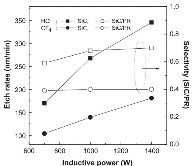
Fig. 2. Measured SiC etch rates and PR selectivity as a function of inductive power for HCl and CF<sub>4</sub> (inductive power: 700–1400 W; bias voltage: –150 V; total gas flow rates: 50 sccm; working pressure: 10 mTorr).
