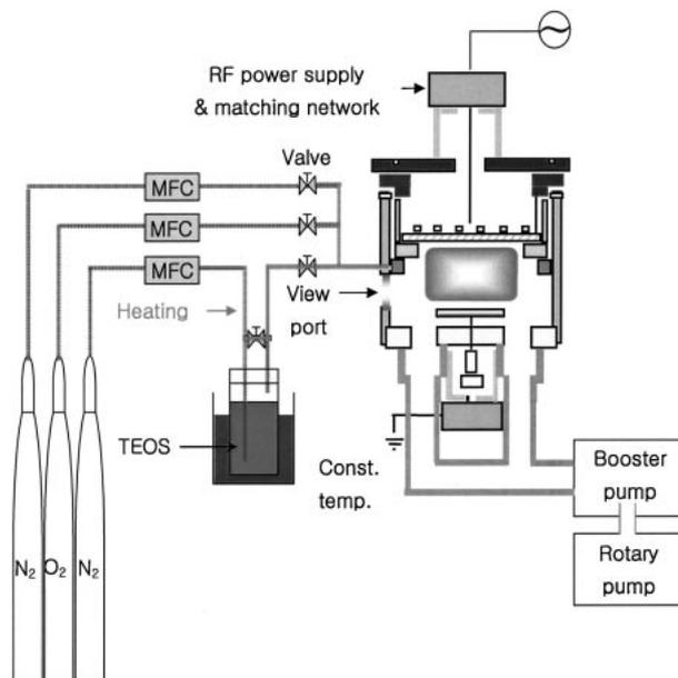
Fig. 1. Schematic diagram of the SiO<sub>2</sub> PECVD system used in the experiment.
