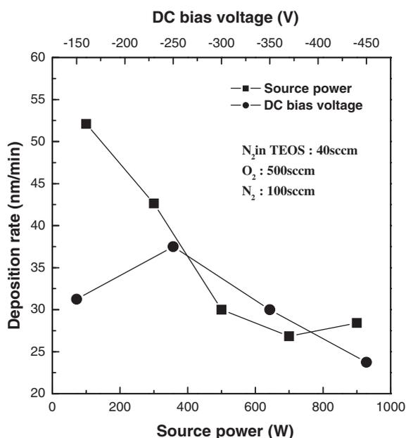
Fig. 2. Deposition rate of the SiO<sub>2</sub> films by PECVD at low temperatures as a function of the source power and dc bias voltage. (condition: N<sub>2</sub> in TEOS 40 sccm, O<sub>2</sub> flow rate 500 sccm, and N<sub>2</sub> flow rate 100 sccm)
