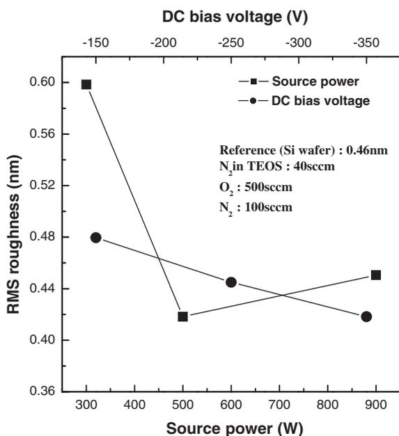
Fig. 3. RMS roughness of the SiO<sub>2</sub> films deposited on a silicon wafer (the roughness is 0.459 nm) as a function of the source power and dc bias voltage measured by AFM. (condition: N<sub>2</sub> in TEOS 40 sccm, O<sub>2</sub> flow rate 500 sccm, and N<sub>2</sub> flow rate 100 sccm)
