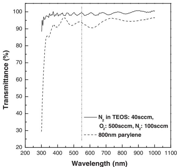
Fig. 6. Optical transmittance of the SiO<sub>2</sub> films deposited by PECVD on a sodalime glass substrate (condition: N<sub>2</sub> in TEOS 40 sccm, O<sub>2</sub> flow rate 500 sccm, N<sub>2</sub> flow rate 100 sccm, source power 500 W, and dc bias voltage -350 V) and the parylene films (800 nm, 20 mTorr) measured by a UV spectrometer. The vertical dash-dotted line indicates a wavelength of 550 nm, which was used as the wavelength for measuring the optical transmittance.
