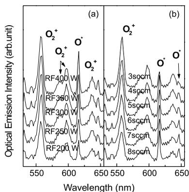
Fig. 1. OES of oxygen plasma in the ion source chamber of the ion gun 2 measured by OES as a function of rf power (a) and oxygen flow rate (b).
