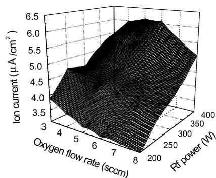
Fig. 2. Variation of the oxygen ion current measured by a Faraday cup as a function of rf power and oxygen flow rate to ion gun 2.
