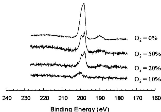
Figure 5. Cl 2p narrow scan spectra at various O<sub>2</sub>-gas mixing ratios.
