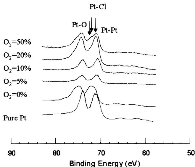
Figure 4. Pt 4f narrow scan spectra at various O<sub>2</sub>-gas mixing ratios.
