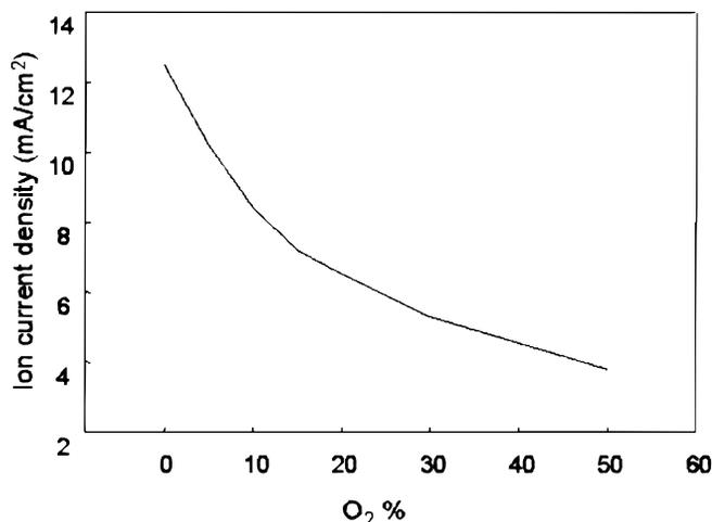
Figure 2. The ion current density with the addition of O<sub>2</sub>.
