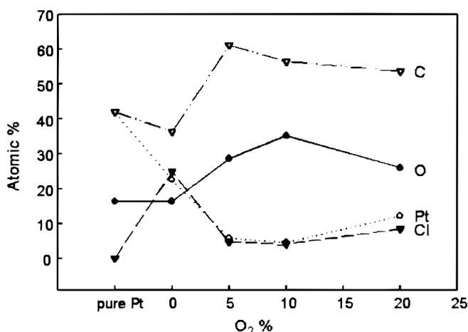
Figure 3. The atomic percent of each element with various O<sub>2</sub>-gas mixing ratios.
