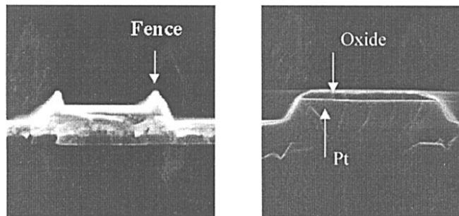
Figure 7. The profile after etch with various gas mixtures: (a, left) 0% O<sub>2</sub> and (b, right) 5% O<sub>2</sub>.
