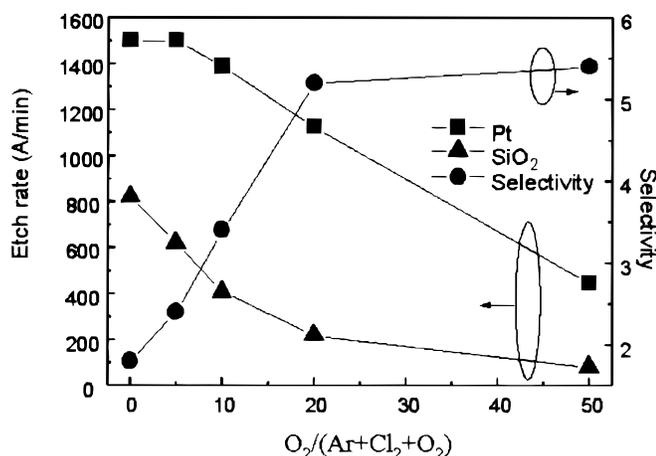
Figure 6. The change of the etch rate and selectivity by the addition of O<sub>2</sub>.
