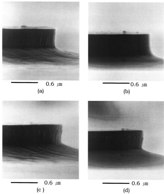
FIG. 3. Etch profiles of different materials used in the GaN laser diode. The materials were etched at 400 V/300 mA ion beam voltage/current, 8 sccm  $\text{Cl}_2$ ,  $50^\circ$  tilt angle, and  $-20^\circ\text{C}$  substrate temperature. (a)  $p$ -GaN, (b) AlGaIn, (c) InGaIn, and (d)  $n$ -GaN.
