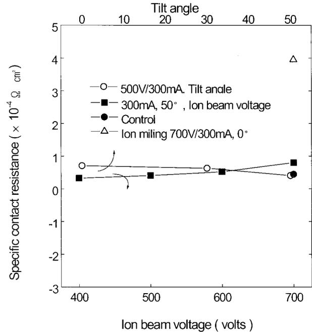
FIG. 7. Effects of ion beam voltage and tilt angle on the ohmic contact resistance of *n*-GaN etched at 300 mA ion beam current and  $-20^{\circ}\text{C}$  substrate temperature.
