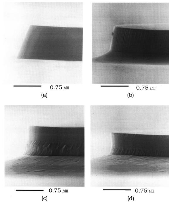
FIG. 2. GaN laser diode etch profile as a function of the tilt angle for 500 V/300 mA ion beam voltage/current, 6 sccm  $\text{Cl}_2$  flow rate, and  $-20^\circ\text{C}$  substrate temperature. (a)  $0^\circ$ , (b)  $30^\circ$ , (c)  $50^\circ$ , and (d)  $60^\circ$ .
