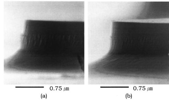
FIG. 4. GaN etch profile etched with 500 V/300 mA Ar ion beam voltage/current,  $50^\circ$  tilt angle,  $-20^\circ\text{C}$  substrate temperature, and (a) 8 and (b) 10 sccm  $\text{Cl}_2$  flow rates.
