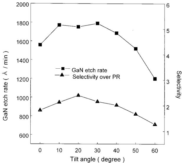
FIG. 1. Angular dependence of the GaN etch rate and the etch selectivity. The angle was measured between the surfaces normal to the substrate and the axis of the ion beam. The Ar ion beam voltage and current were 500 V and 300 mA, respectively, the  $\text{Cl}_2$  flow rate was 6 sccm, and the substrate temperature was  $20^\circ\text{C}$ .
