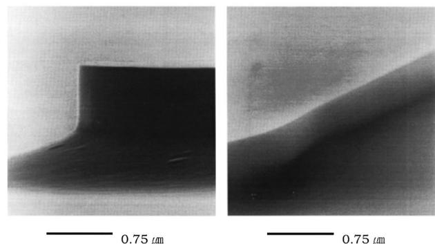
FIG. 5. GaN etch profile etched under the optimized conditions of Ar ion beam voltage/current and  $\text{Cl}_2$  flow rate.
