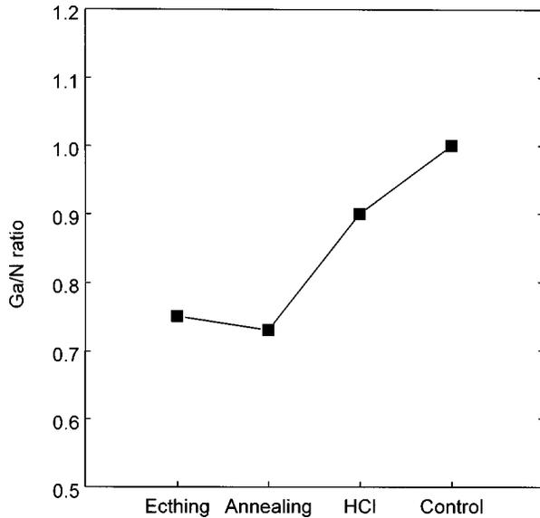
FIG. 6. Ga/N ratio of the etched GaN surface measured by XPS. Etch conditions: Ar ion beam condition/current 500 V/300 mA, tilt angle 50°, substrate temperature  $-20^{\circ}\text{C}$ , and  $\text{Cl}_2$  6 sccm flow rate.
