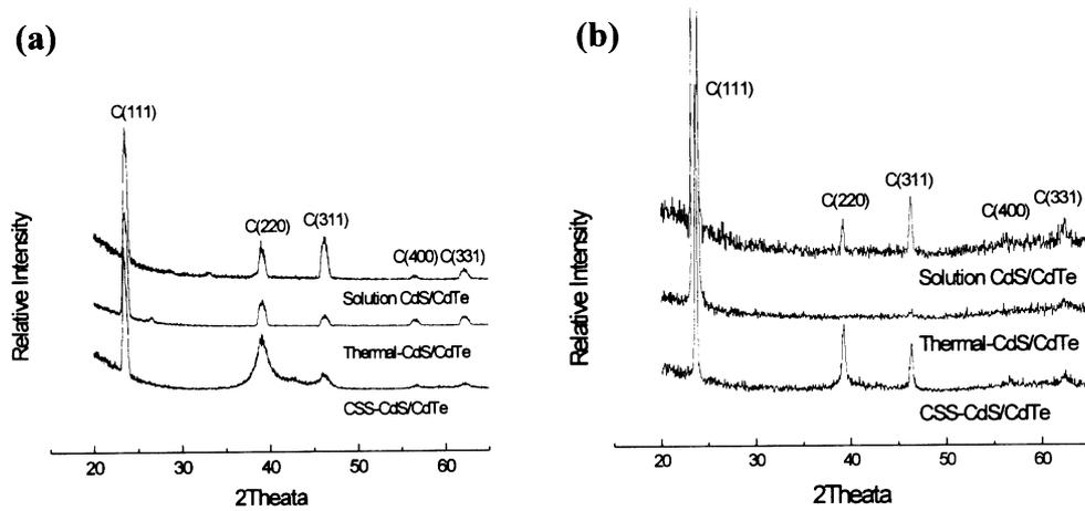
Fig. 2. X-ray diffraction data of CdTe thin films deposited on the variously prepared CdS thin films. CdTe thin films were annealed at 550°C using rapid thermal annealing (a) and at 400°C using furnace annealing after the treatment in  $\text{CdCl}_2 + \text{CH}_3\text{OH}$  solution (b).
