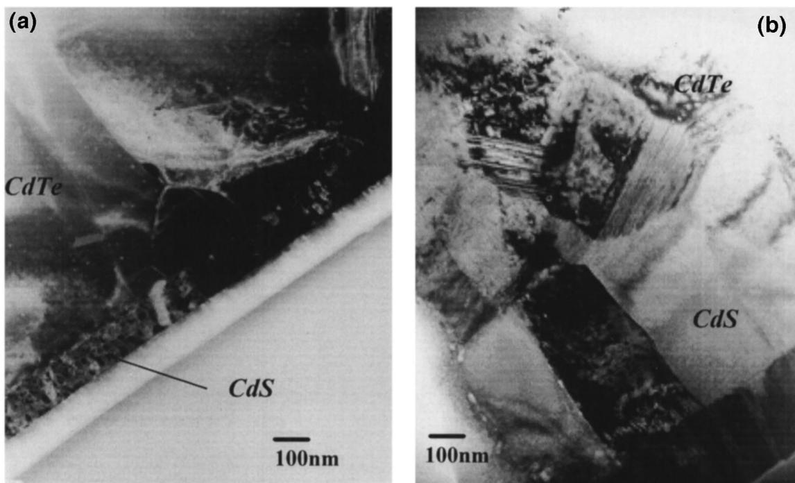
Fig. 3. Cross-sectional TEM micrographs of the furnace annealed CdTe/Solution grown CdS (a) and the CdTe/CSS grown CdS (b).
