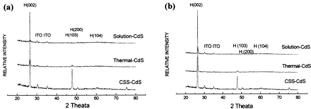
Fig. 1. X-ray diffraction data of CdS thin films deposited variously (a) and annealed thin films in the  $H_2$  environment (b).
