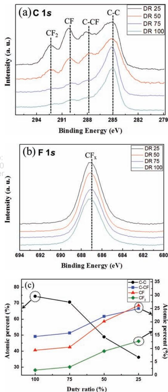
**Figure 5.** XPS narrow scan data of (a)  $C 1s$  and (b)  $F 1s$  of the ACL surfaces etched with  $O_2/CHF_3$ , and (c) relative percentages of the different carbon binding states such as C-C, C-CF, CF and  $CF_2$  deconvoluted from (a).
