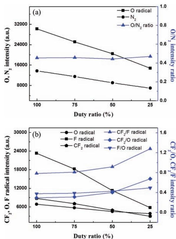
**Figure 3.** Change of the radical intensities in (a)  $O_2/N_2$  plasmas and (b)  $O_2/CHF_3$  plasmas measured using OES as a function of pulse duty.
