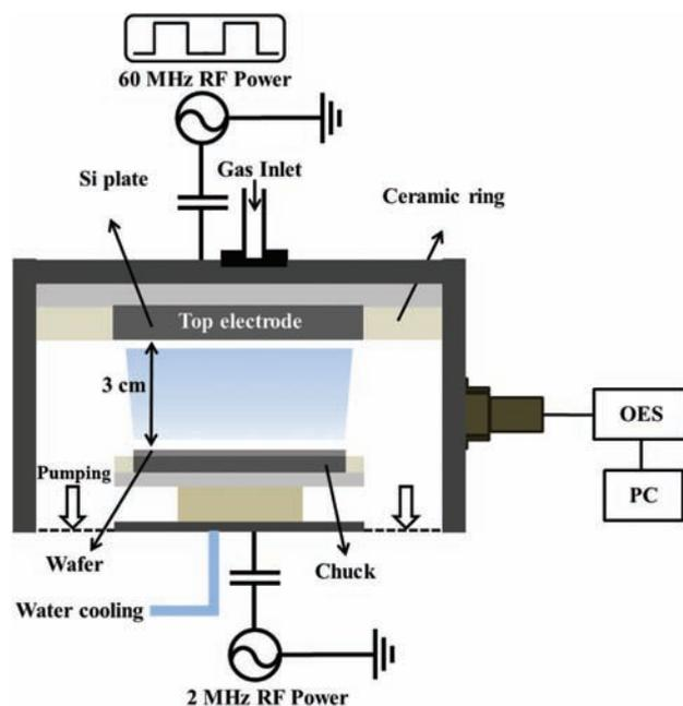
**Figure 1.** The 60/2 MHz pulsed DF-CCP system used in this study. The 60 MHz rf power was pulsed at 1 kHz of pulse frequency with the duty percentage from 100% (continuous wave: CW) to 25%. A continuous wave 2 MHz rf power was applied to the substrate while keeping the same average bias voltage.
