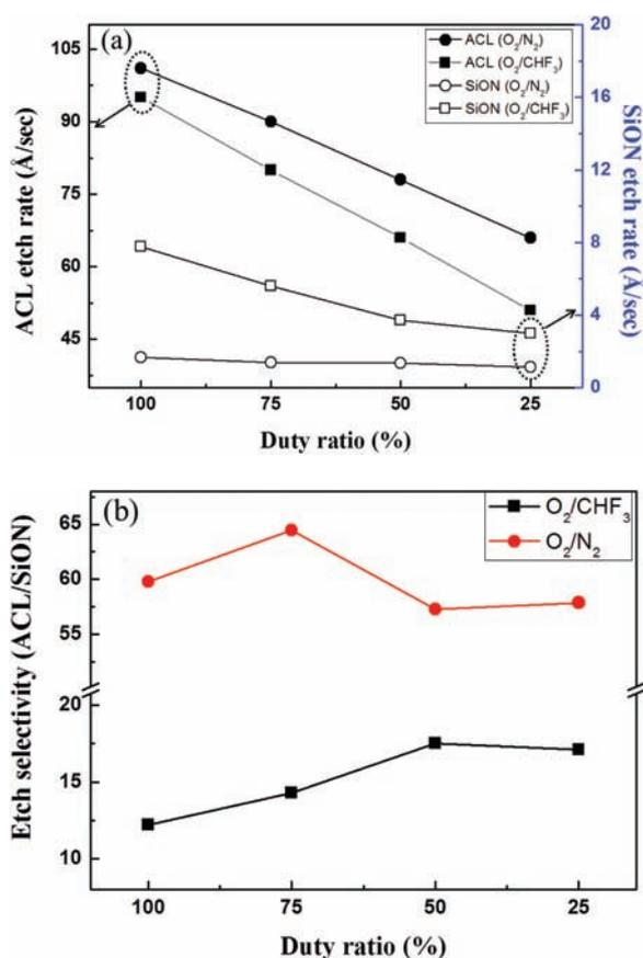
**Figure 2.** Effects of rf source power pulsing on (a) the etch rates of ACL and SiON, and (b) the etch selectivities of ACL/SiON for the gas mixtures of  $O_2/N_2$  (40/60 sccm) and  $O_2/CHF_3$  (40/60 sccm).
