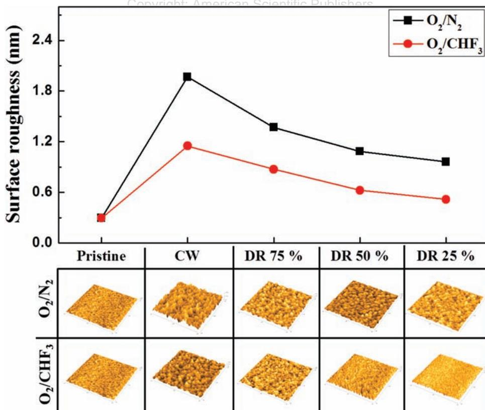
**Figure 6.** Surface roughness of the ACL after etching with  $O_2/N_2$  and  $O_2/CHF_3$ , measured using AFM as a function of pulse duty percentage.
