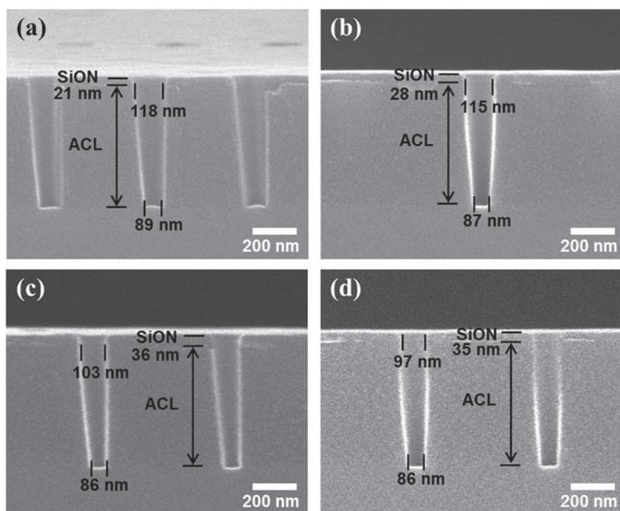
**Figure 8.** Etch profiles of 600 nm thick ACL masked with SiON etched with  $O_2/CHF_3$  at different pulse duty percentages of (a) 100%, (b) 75%, (c) 50%, and (d) 25%.
