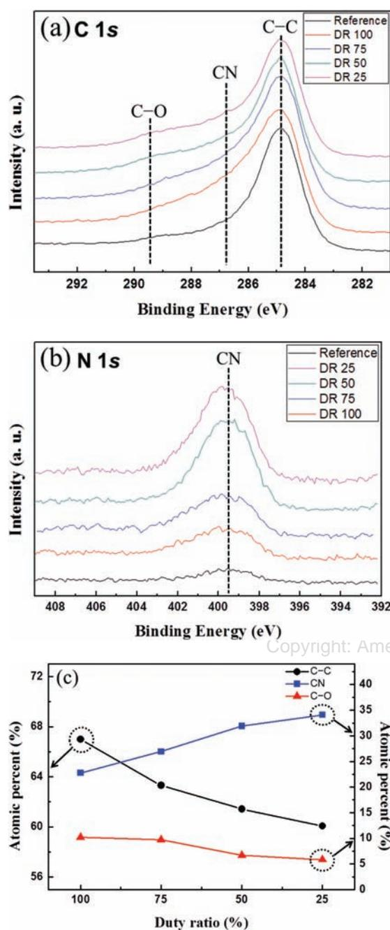
**Figure 4.** XPS narrow scan data of (a)  $C 1s$  and (b)  $N 1s$  of the ACL surfaces etched with  $O_2/N_2$ , and (c) relative percentages of the different carbon binding states such as C-C, CN, and C-O deconvoluted from (a).
