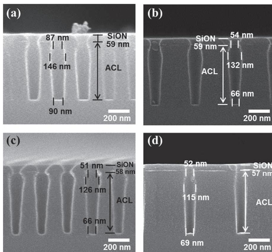
**Figure 7.** Etch profiles of 600 nm thick ACL masked with SiON etched with  $O_2/N_2$  at different pulse duty percentages of (a) 100%, (b) 75%, (c) 50%, and (d) 25%.
