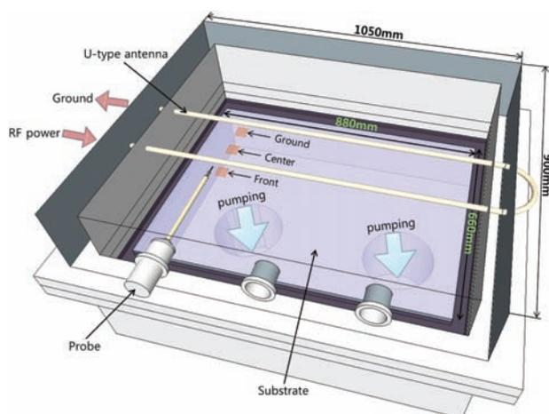
**Figure 1.** Schematic diagram of the ICP source used in the experiment.
