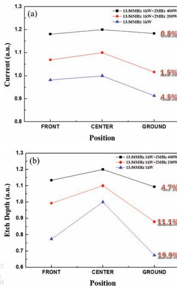
**Figure 4.** (a) Variation of ion saturation current measured using an electrostatic probe across the U-type antenna as a function of 2 MHz rf power while maintaining 1 kW of 13.56 MHz to estimate the plasma uniformity. Ar 200 mTorr was used. (b) Etch depth of photoresist as a function of 2 MHz rf power while maintaining 1 kW of 13.56 MHz. The photoresist was etched using 200 mTorr of Ar/O<sub>2</sub> (8:2).
