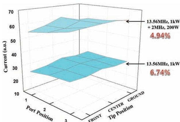
**Figure 5.** Uniformity of ion saturation current measured using an electrostatic probe over the area covered by the U-shaped antenna. The ion saturation current was measured for the single frequency of 1 kW 13.56 MHz only and for the dual frequency of 1 kW 13.56 MHz + 0.2 kW 2 MHz. As the operating condition, 200 mTorr of Ar was used.
