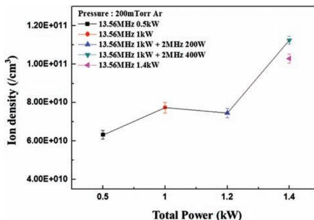
**Figure 2.** Ion density as a function rf power for 13.56 MHz only and for the dual frequency composed of 13.56 MHz and 2 MHz measured using the Langmuir probe. The plasmas were generated using 200 mTorr of Ar.
