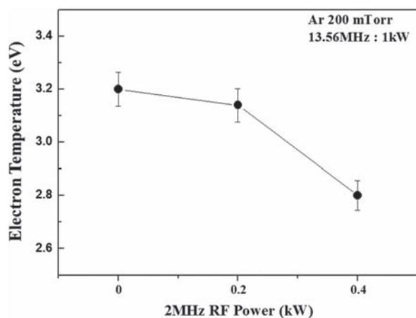
**Figure 3.** Electron temperature measured for the dual frequency rf power as a function of 2 MHz rf power while maintaining 1 kW of 13.56 MHz.
