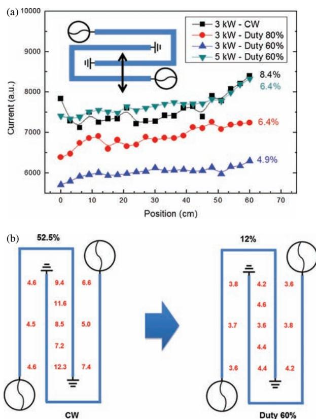
**Figure 5.** (a) Plasma non-uniformity measured by ion saturation current probe and (b) SiO<sub>2</sub> etch non-uniformity at CW and 60% of rf pulse duty percentage of 3 kW rf power without biasing the substrate. In (a), plasma uniformity measured at 5 kW and 60% duty percentage was also included to compare with 3 kW CW condition as the same average rf power of 3 kW.
