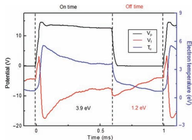
**Figure 2.** Instant plasma potential ( $V_p$ ) and the instant floating potential ( $V_f$ ) measured as a function of operation time using an emissive probe for 5 kW of rf power to the ICP power and 60% rf duty percentage. As the operating gas, 10 mTorr of CF<sub>4</sub> gas was used. The instant electron temperature calculated from the instant  $V_p$  and the instant  $V_f$  is also shown.
