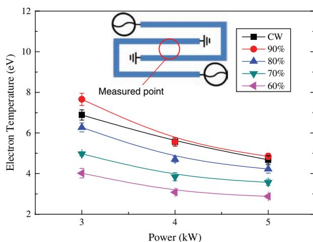
**Figure 3.** Electron temperature estimated by an emissive probe as a function of pulse condition for  $\text{CF}_4$  plasma.
