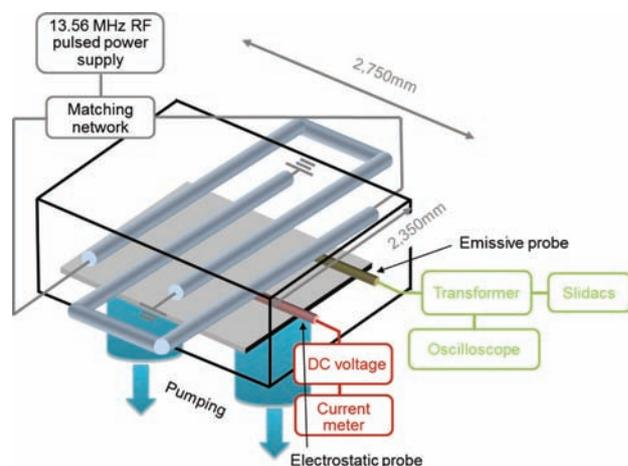
**Figure 1.** Schematic diagram of an internal-type linear ICP system, a homemade emissive probe and an electrostatic probe used in this experiment.
