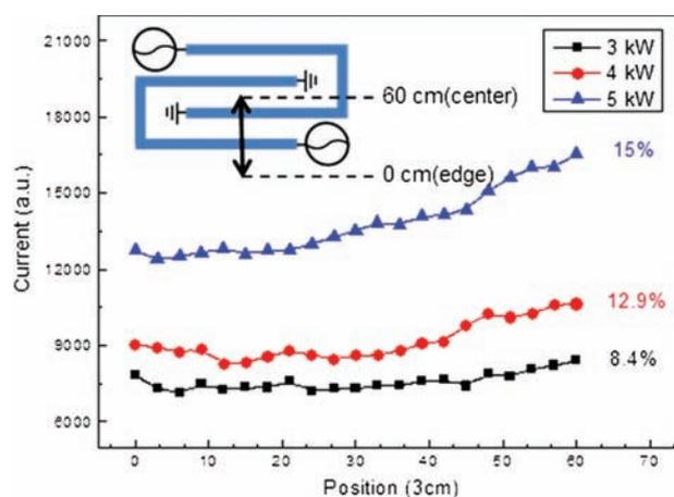
**Figure 4.** Plasma non-uniformity measured by an electrostatic probe as a function of CW rf power at  $\text{CF}_4$  plasma.
