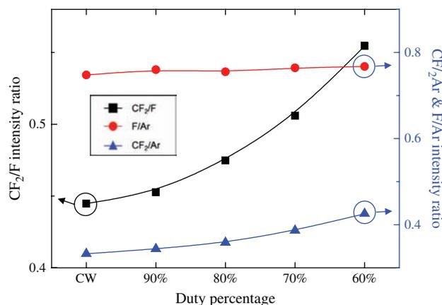
**Figure 6.** Relative concentrations of CF<sub>2</sub> (I<sub>CF<sub>2</sub></sub>/I<sub>Ar</sub>) and F (I<sub>F</sub>/I<sub>Ar</sub>) measured by OES using Ar actinometry. The concentration ratio CF<sub>2</sub>/F ratio measured as a function of pulse duty percentage at the gas mixture of an Ar/CF<sub>4</sub> (1:9) was also included.
