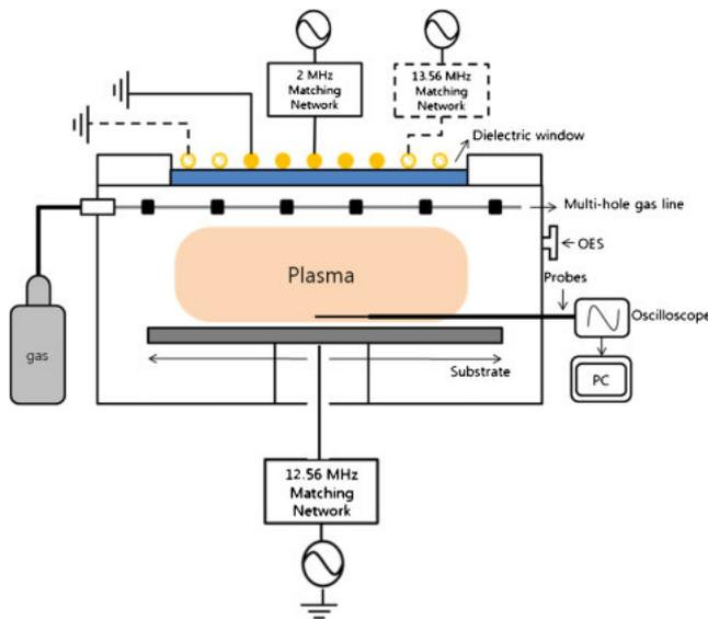
**Fig. 1.** (Color online) Schematic diagram of the DF-ICP system used in this experiment.
