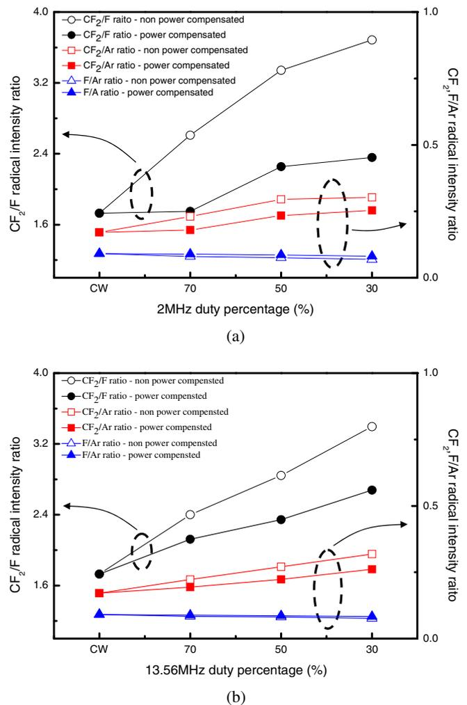
**Fig. 4.** (Color online) Optical emission intensity ratio of F/Ar, CF<sub>2</sub>/Ar, and CF<sub>2</sub>/F measured as a function of pulse duty percentage of (a) 2 MHz rf power or (b) 13.56 MHz rf power for both the rf power compensated and non-compensated modes. An Ar/C<sub>4</sub>F<sub>8</sub> (10 : 2) gas mixture at 10 mTorr was utilized in this experiment. The other operating conditions were the same as those in Figs. 2(a) and 3(a), respectively.
