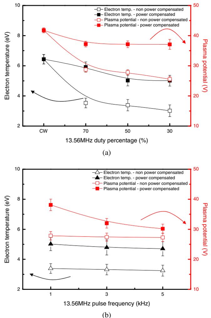
**Fig. 3.** (Color online) Plasma potential and electron temperature as a function of (a) pulse duty percentage at the pulse frequency of 5 kHz and (b) pulse frequency at the duty percentage of 50% for the rf power compensated and non-compensated modes. The 13.56 MHz rf power was pulsed from CW conditions (800 W) to 30% while keeping the 2 MHz rf power provided to the inner antenna at CW conditions (300 W). The other operating conditions were the same as those in Fig. 2.
