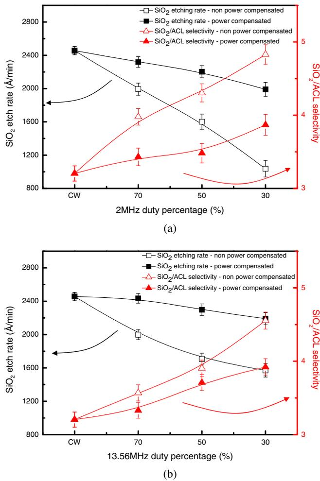
**Fig. 5.** (Color online) Etch rates of SiO<sub>2</sub> and the etch selectivities of SiO<sub>2</sub> over ACL measured as a function of (a) 2 MHz rf power duty percentage and (b) 13.56 MHz rf power duty percentage for the rf power compensated and non-compensated modes. The substrate was biased at  $-100$  V using a separate 12.56 MHz rf power source while maintaining the substrate at room temperature. The other operating conditions were the same as those in Fig. 4.
