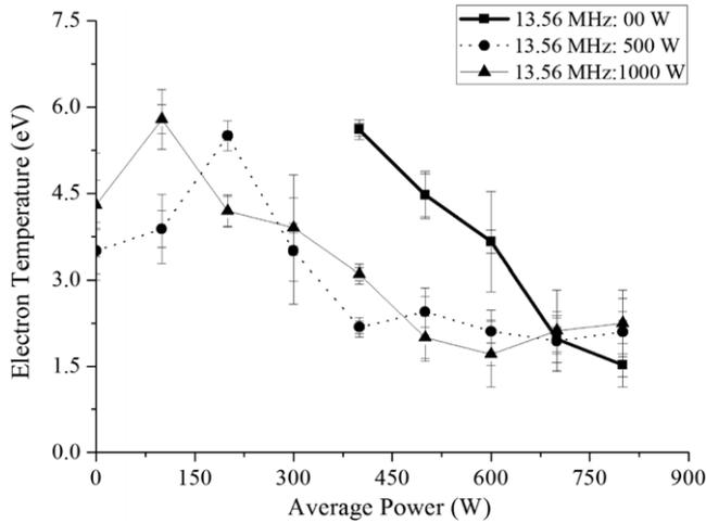
**Figure 4.** Electron temperature variation with 2 MHz RF power for three different 13.56 MHz RF powers.
