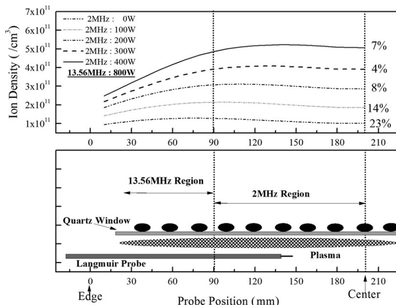
Figure 6. Ion flux density distribution over the substrate surface area and a schematic of Langmuir probe measurement region.
