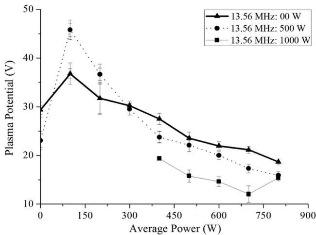
**Figure 5.** Plasma potential variation with 2 MHz RF power for three different 13.56 MHz RF powers.
