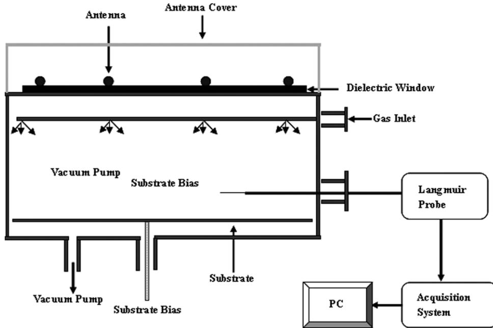
**Figure 2.** Schematic diagram of the experimental set-up with data acquisition arrangement. The Langmuir probe was located at 70 mm below the antenna (near substrate region) and 60 mm away from the centre of the antenna.
