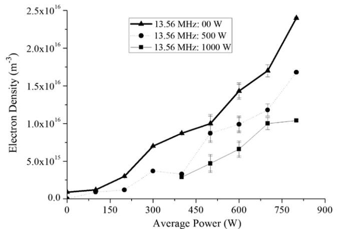
**Figure 3.** Electron density variation in the plasma with 2 MHz RF power for three different 13.56 MHz RF powers.
