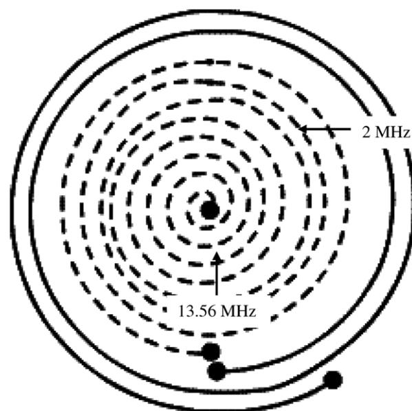
**Figure 1.** Schematic of dual frequency inductively coupled antenna. The inner coil (shown by a broken line) was used to feed 2 MHz RF power, whereas the outer coil (shown as a solid line) was fed by 13.56 MHz RF power.
