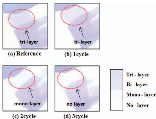
**Figure 4.** Optical images of exfoliation graphene on  $SiO_2/Si$  measured as a function of ALET cycles. (a) trilayer graphene before ALET of graphene ( $Si/SiO_2(300\text{ nm})/graphene$ ) (b) After 1 cycle ALET, bilayer graphene surface after the removal of one layer graphene (c) After 2 cycle ALET, monolayer graphene surface after the removal of two graphene layers. (d) After 3 cycle ALET, no graphene on  $Si/SiO_2$  after the removal of three layers of graphene.
