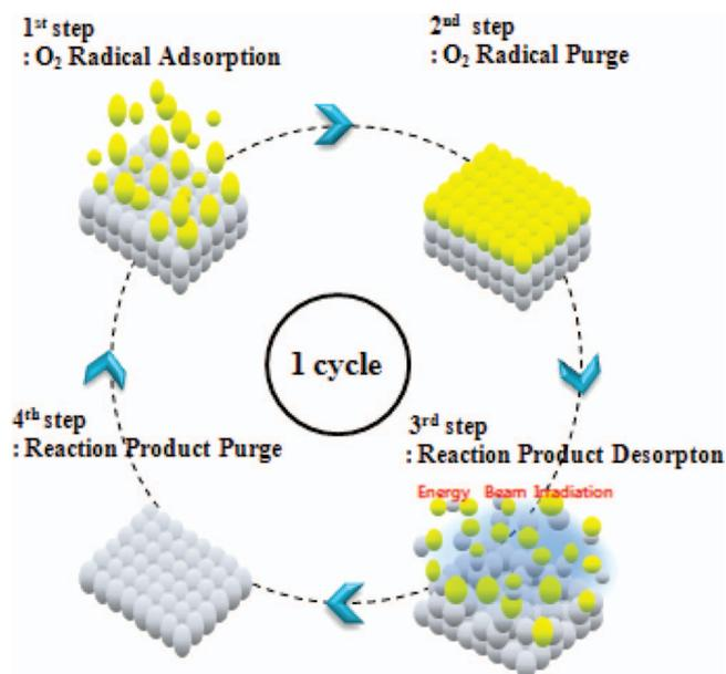
Figure 1. Concept of four step graphene ALET cycle.
