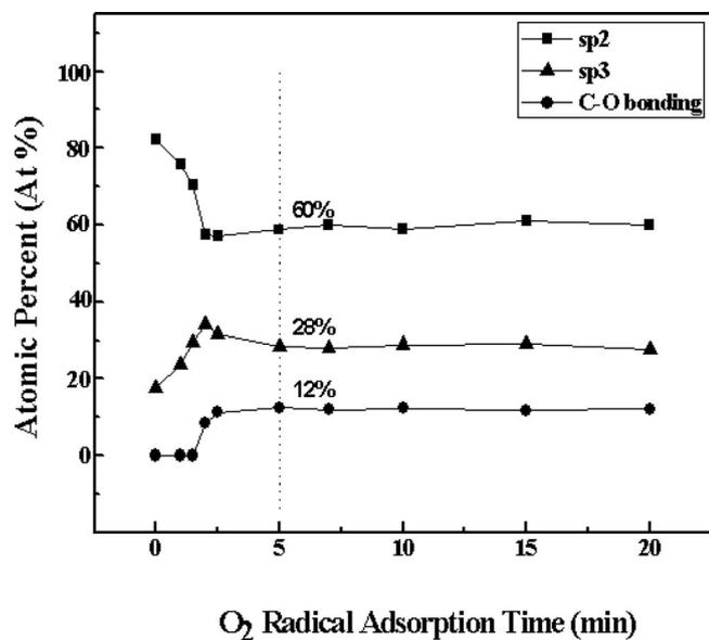
**Figure 3.** Atomic percentage (%) of carbon bondings ( $sp^2$ ,  $sp^3$ , and C-O) on the HOPG surface measured after the chemical adsorption step as a function of  $O_2$  radical exposure time by XPS at the take off angle of  $60^\circ$ .
