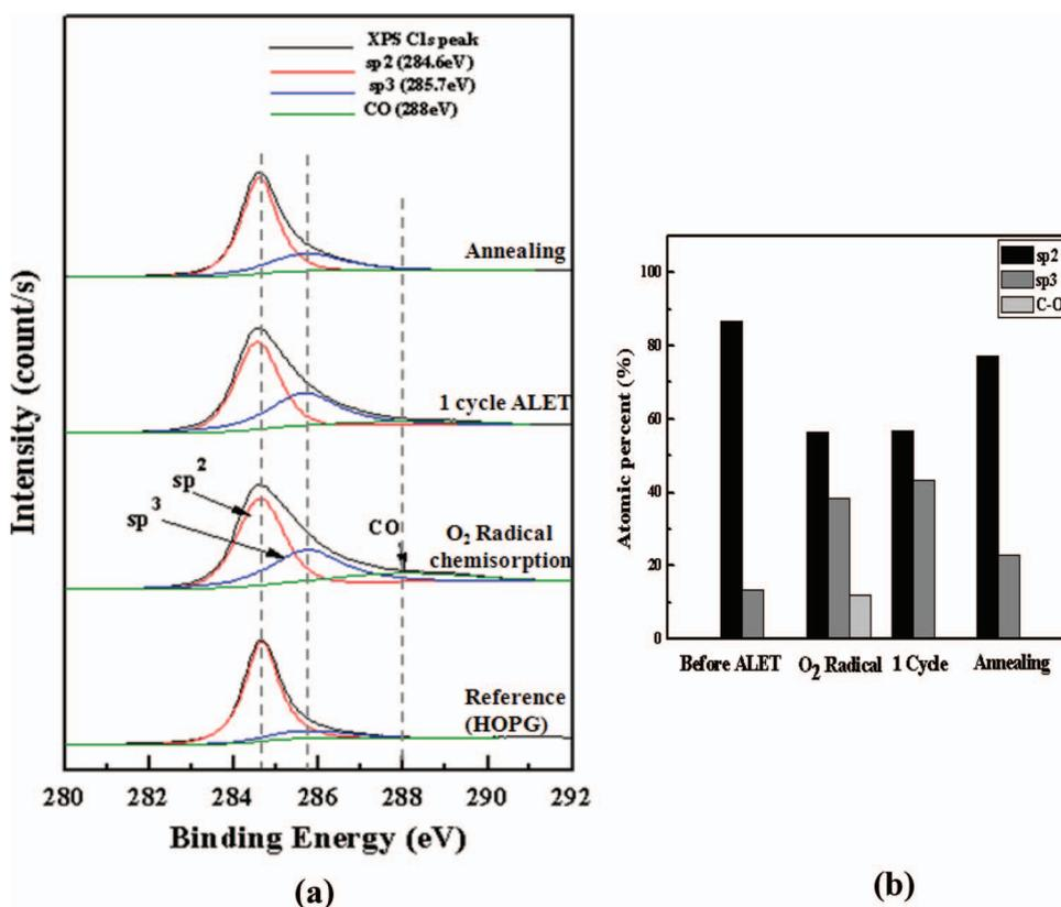
Figure 2. (a) XPS C1s data of HOPG surface after each step of the etch cycles (reference, after oxygen chemisorption, after 1 cycle ALET, and after annealing). (b) Atomic percentage (%) of carbon bondings ( $sp^2$ ,  $sp^3$ , and C-O) on the HOPG surfaces obtained after the deconvolution of the XPS C1s data in Figure 2a. Observed graphene surface was measured by XPS at the take off angle of 60°.
