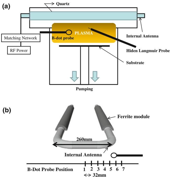
**Fig. 1** **a** Schematic diagram of the ICP system with the ferrite module used in the experiment. **b** Arrangement of the internal antenna with the ferrite module used in the experiment
