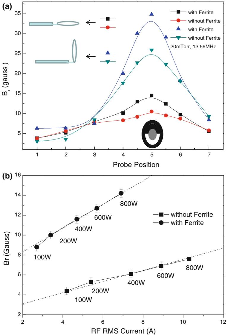
**Fig. 3** **a** The induced magnetic field  $B$  measured by a B-dot probe at 10 mm under the antenna with/without ferrite module. **b** The magnetic field measured just below the antenna as a function of antenna current for the ICP with and without the ferrite module
