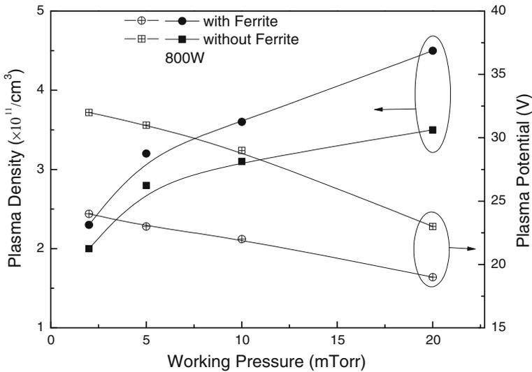
**Fig. 6** Plasma density and plasma potential measured by a Langmuir probe at 4 cm below the antenna as a function of pressure at 800 W of rf power
