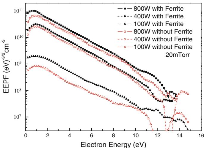
**Fig. 4** EEPFs of the Ar plasmas at 20mTorr measured as a function of rf power for the ICPs with and without ferrite module
