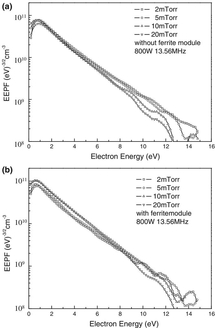
**Fig. 5** EEPFs of the Ar plasmas at 800 W measured as a function of pressure for the ICPs **a** without and **b** with the ferrite module
