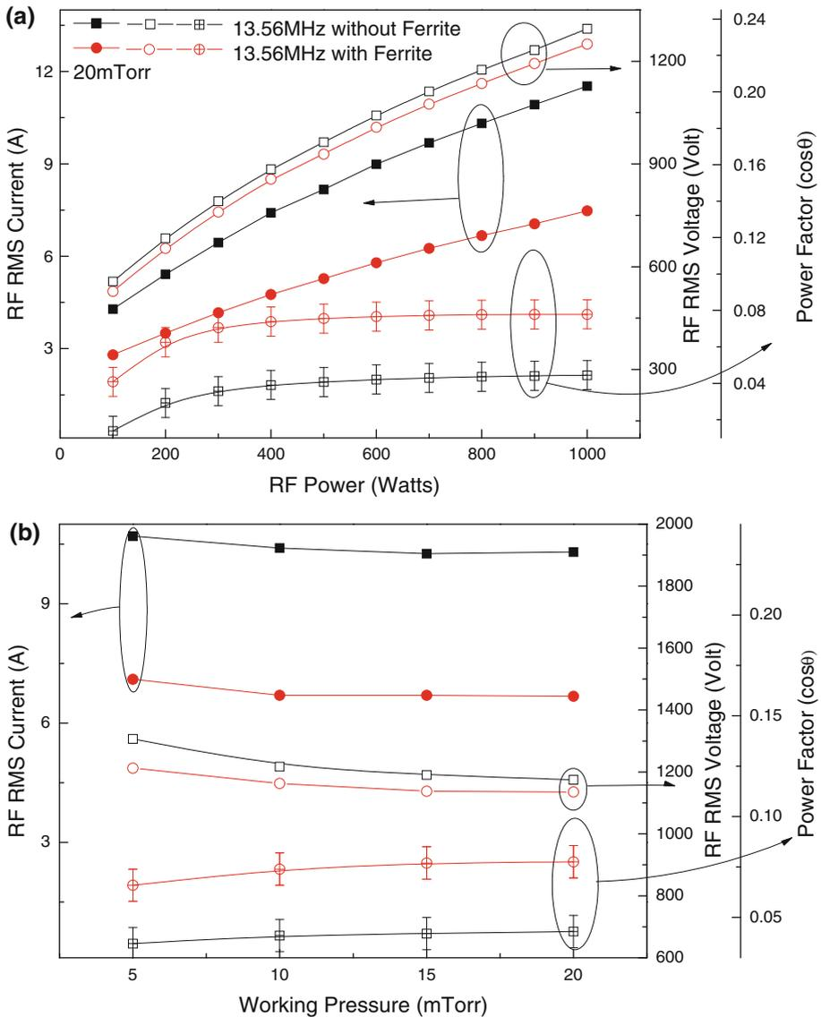
**Fig. 2** Rf rms voltage and current measured **a** as a function of rf power at 20mTorr Ar and **b** as a function of operating pressure at 800 W of rf power for the internal ICP source with/without the ferrite module by an impedance analyzer on the antenna located close to the rf power input
