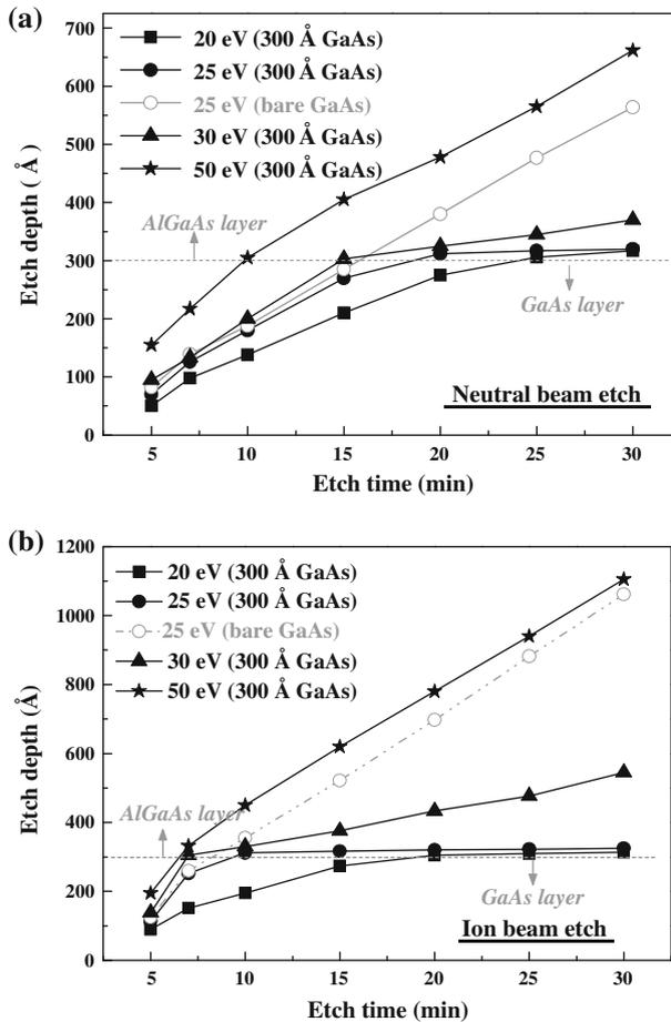
**Fig. 1** Etch depth of bare GaAs and 300 Å GaAs on AlGaAs **a** by the  $\text{Cl}_2/\text{O}_2$  neutral beam and **b** by the  $\text{Cl}_2/\text{O}_2$  ion beam as a function of etch time
