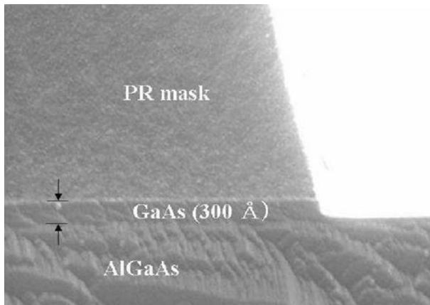
**Fig. 2** SEM etch profile after the etching of 300 Å GaAs on AlGaAs using  $\text{Cl}_2/\text{O}_2$  neutral beam with +25 V of the first grid voltage
