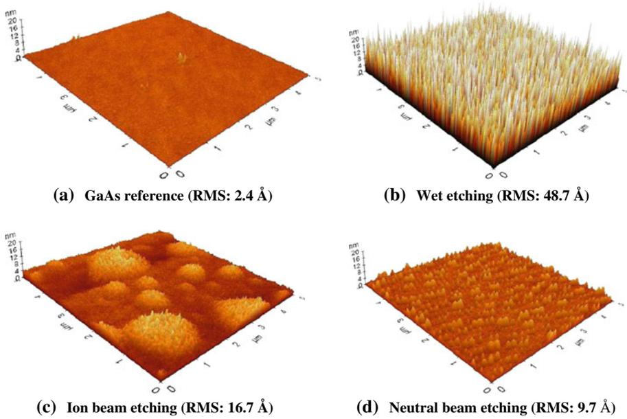
**Fig. 4** Surface roughness on AlGaAs surfaces evaluated by AFM after the removal of 300 Å GaAs on AlGaAs
