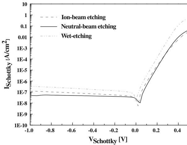
**Fig. 5** I-V characteristics of the Schottky diode fabricated after the wet etching, ion beam etching and neutral beam etching
