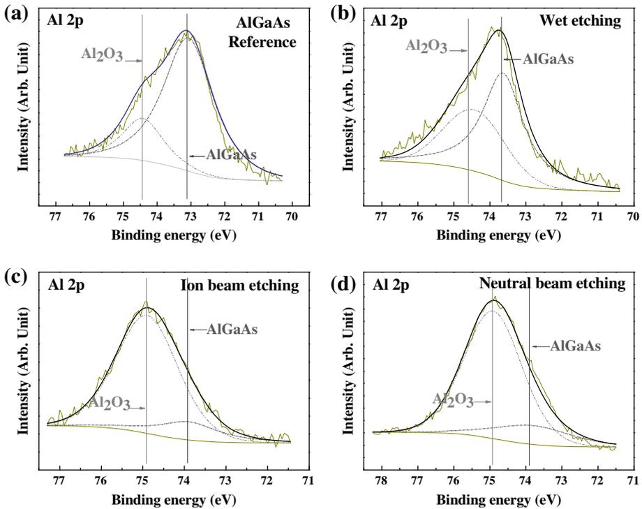
**Fig. 3** The XPS narrow scan data related to Al atomic peak of AlGaAs surface before and after the etching of AlGaAs. **a** AlGaAs reference **b** Wet etching **c** Ion beam etching **d** Neutral beam etching
