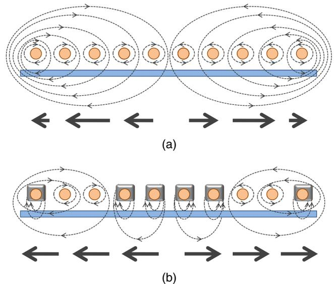
Fig. 5. (Color online) Schematic drawing of the induced magnetic field by the spiral ICP antenna for (a) without and (b) with ferrite modules installed locally at the center and edge of the antenna.
