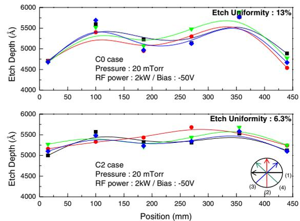
Fig. 6. (Color online) The etch uniformity of SiO<sub>2</sub> measured at the RF power of 2000 W, dc bias voltage of -50 V, and a C<sub>2</sub>F<sub>6</sub> pressure of 20 mTorr.
