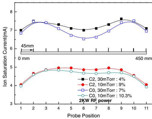
Fig. 4. (Color online) Plasma uniformities of the C0 and C2 antennas measured using a movable Langmuir probe system as a function of operating pressure at the rf power of 2000 W.
