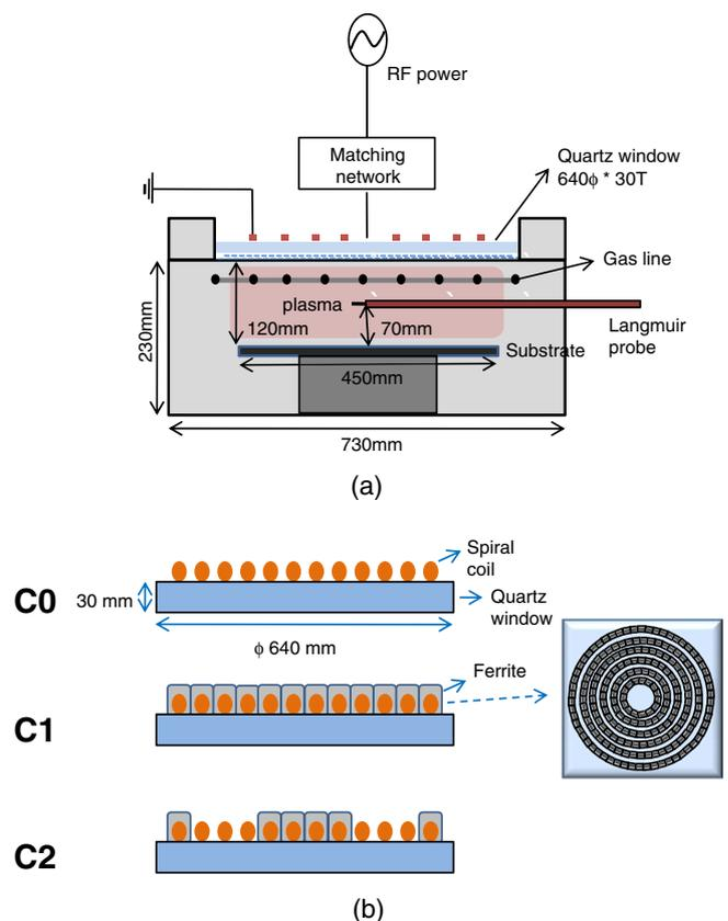
Fig. 1. (Color online) (a) Schematic diagram of 450 mm inductively coupled plasma system. (b) Three different antenna configurations with and without ferrite modules.
