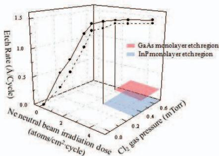
Figure 2. III-V compound materials ALET process window measured as a function of the Cl<sub>2</sub> gas pressure and Ne neutral beam irradiation dose. The Ne beam energy measured before the reflection to the reflector was 32 V. This figure was made from the data from the reference 11, 13 shown below.
