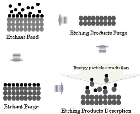
Figure 1. Concept of the ALET Process. This figure was made from the data from the reference [1] shown below.
