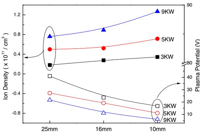
**Fig. 2.** (Color online) Ar<sup>+</sup> plasma density and plasma potential measured using a Langmuir probe at the center of the chamber for inner antenna diameters of 10, 16, 25 mm and RF powers of 3, 5, and 9 kW at 5 mTorr Ar.
