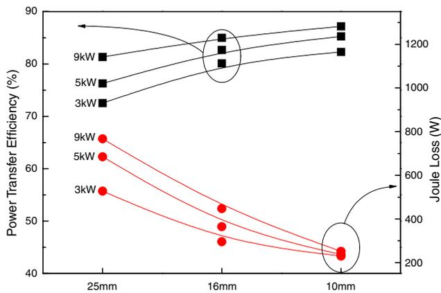
**Fig. 4.** (Color online) Joule loss and power transfer efficiency for antenna diameters of 10, 16, 25 mm and RF powers of 3, 5, and 9 kW at 5 mTorr Ar measured by an impedance analyzer.
