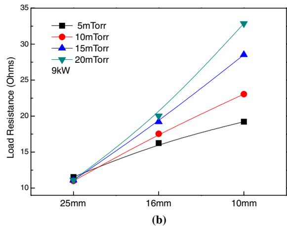
**Fig. 3.** (Color online) Load resistance measured as a function of (a) RF power and (b) working pressure, for inner antenna diameters of 10, 16, 25 mm, by an impedance analyzer on the antenna located close to the RF power input.
