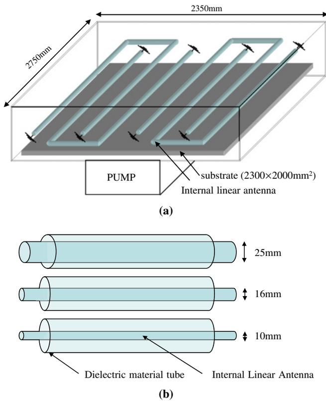
**Fig. 1.** (Color online) (a) Schematic diagram of the large area, internal-type, linear inductively coupled plasma source used in this study. (b) Arrangement of the internal-type linear antennas, where, 10, 16, and 25 mm inner antenna diameters were enclosed by the same size dielectric tubing.
