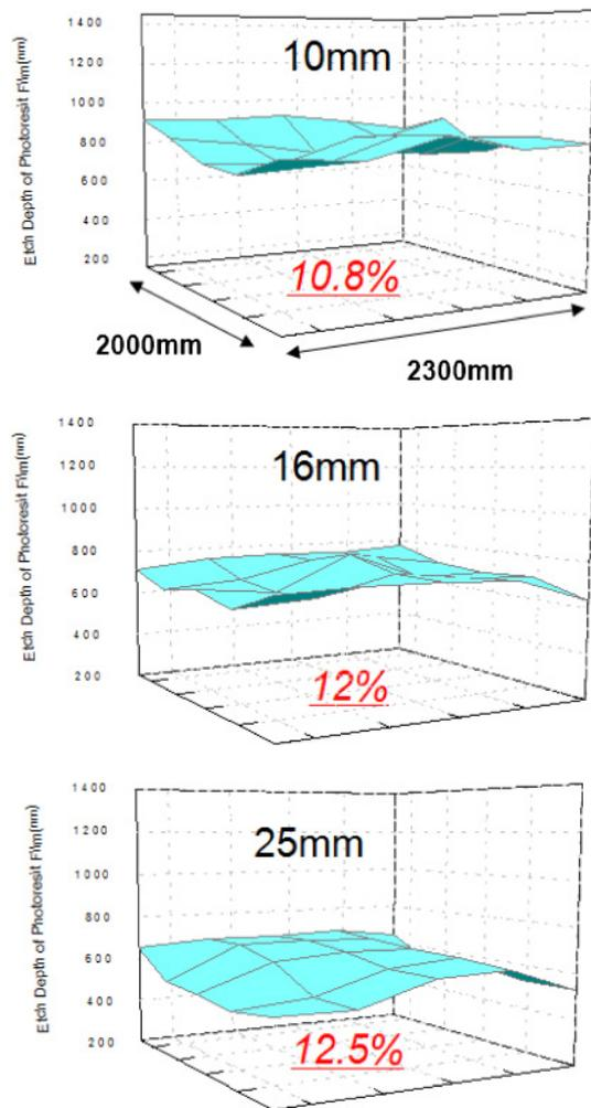
**Fig. 5.** (Color online) Etch uniformity of photoresist film on a substrate area of 2,300 × 2,000 mm<sup>2</sup> measured at an RF power of 8 kW and with an Ar : O<sub>2</sub> (7 : 3) mixture gas for antenna diameters of 10, 16, and 25 mm at 15 mTorr Ar.
