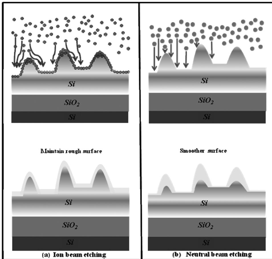
**Figure 5.** Top silicon etch mechanism of the SOI wafer by (a) an ion beam and (b) a neutral beam.
