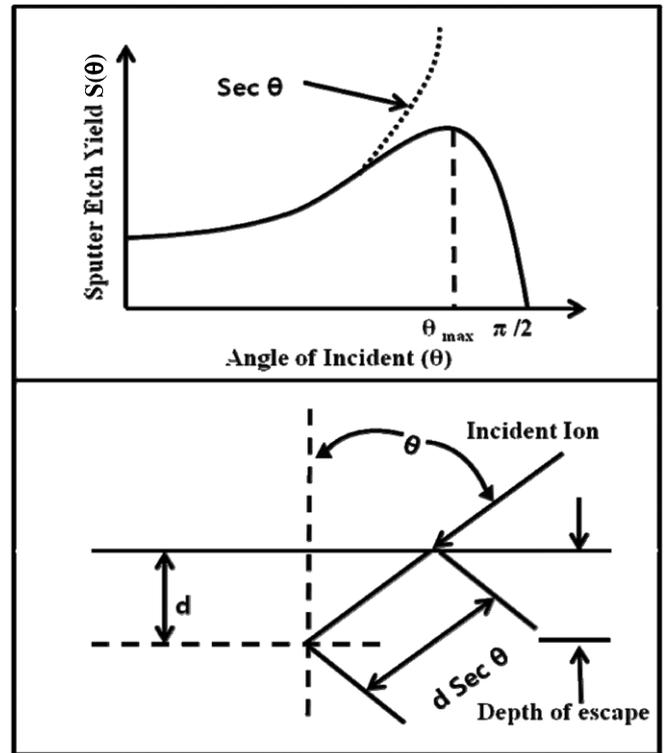
**Figure 4.** Sputter etch yield versus incident angle of the bombarding particle.
