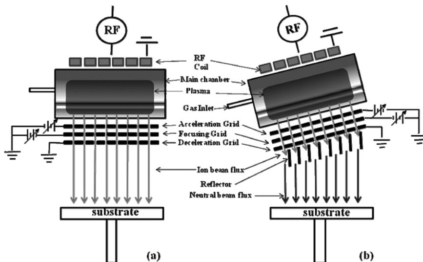
**Figure 1.** Schematic diagram of (a) the ICP-type ion beam etching system and (b) the low-angle forward-reflected neutral beam etching system used in the experiment.
