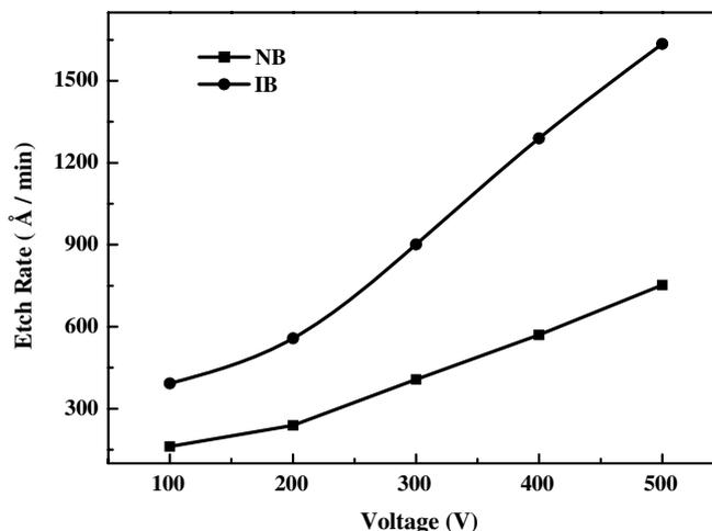
**Figure 2.** Etch rates of the top silicon layer of the SOI wafer for the neutral beam (NB) etching and the ion beam (IB) etching measured as a function of the first grid voltage (~particle beam energy) at 15 sccm of Cl<sub>2</sub>.
