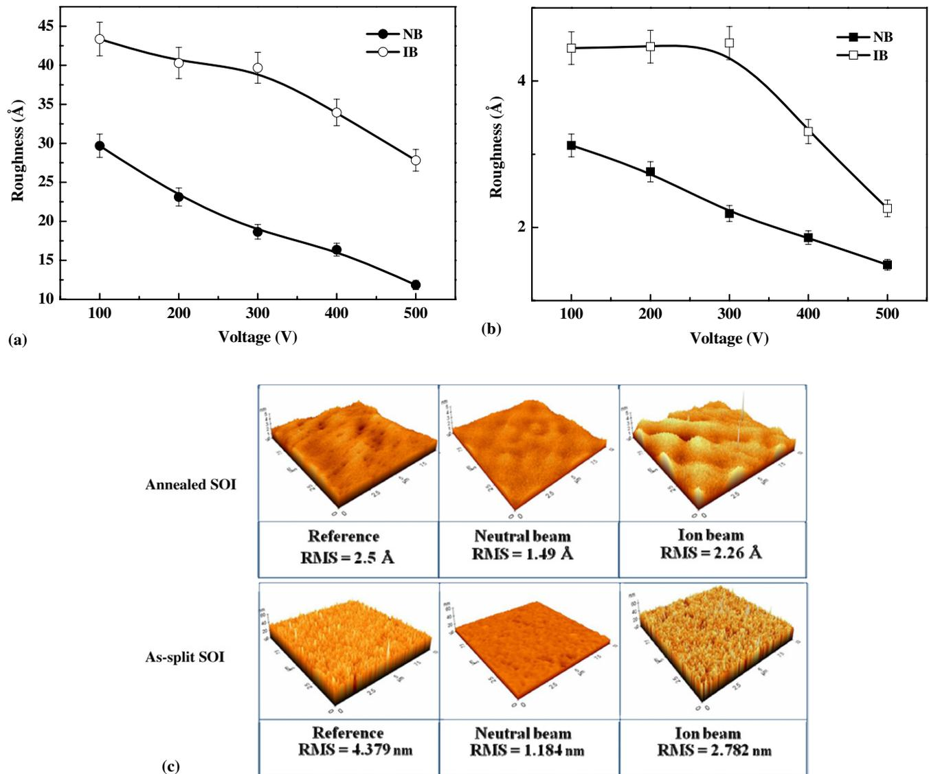
**Figure 3.** The rms surface roughness measured on the 100 nm-thick remaining top silicon after the etching of (a) the as-split annealed SOI wafer (before the etching, the rms roughness of 300 nm-thick top silicon layer was 43.79 Å) and (b) the annealed SOI wafer (before the etching, the rms roughness of the 270 nm-thick top silicon layer was 2.5 Å). (c) shows the AFM images of SOI wafer surfaces before/after etching with the first grid voltage of 500 V.
