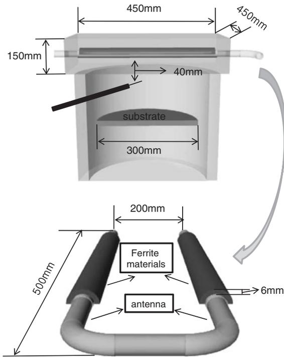
Fig. 1. Schematic diagram of FE-ICP system used in the experiment.
