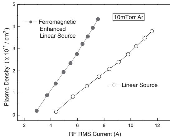
Fig. 3. Ar<sup>+</sup> ion density measured by a Langmuir probe at 4 cm below the antenna as a function of RF rms current for the ICP source with/without the ferromagnetic material. The operation pressure was maintained at 10 mTorr.
