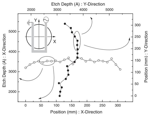
Fig. 5. Etch depth of the PR over a substrate area of 300mm wafer measured at 600 W of RF power and 10 mTorr of operating pressure in an Ar/O<sub>2</sub> (9 : 1) mixture.
