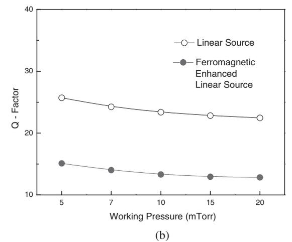
Fig. 4. Quality factor calculated with the data obtained by an impedance probe (a) as a function of RF power at 10 mTorr Ar and (b) as a function of working pressure at 600 W of RF power for the ICP system with/without the ferromagnetic material.
