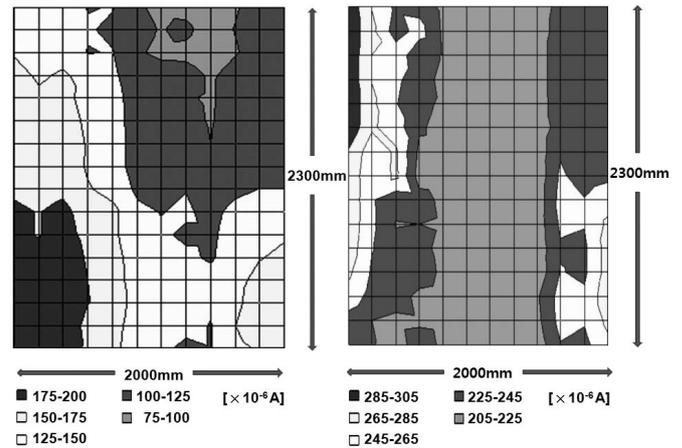
Fig. 6. Uniformity of the ion saturation current of the serpentine-type antenna and the double-comb-type antenna over a substrate area of 2,300 mm  $\times$  2,000 mm measured by using a movable electrostatic probe having 12 tips biased at  $-65$  V for 15 mTorr of Ar and the rf power of 4.5 kW.
