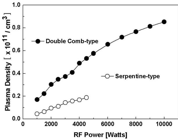
Fig. 5. Plasma density of the serpentine-type antenna and the double-comb-type antenna measured using a Langmuir probe as a function of rf power at 15 mTorr Ar.
