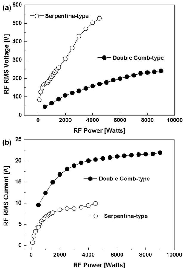
Fig. 3. (a) rf rms voltage and (b) rf rms current on the serpentine-type antenna and double-comb-type antenna measured as a function of the rf power at 15 mTorr Ar.
