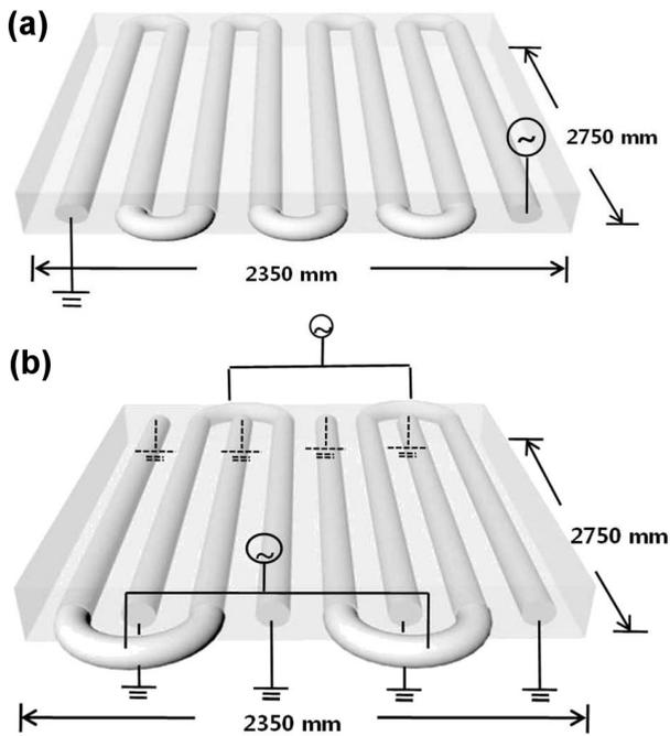
Fig. 1. Schematic diagrams of (a) serpentine-type antenna and (b) double-comb-type antenna used in the experiment.
