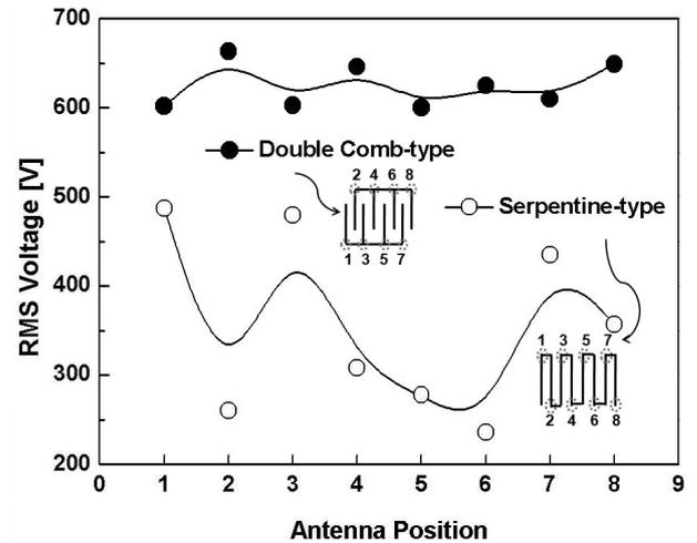
Fig. 2. Rf rms voltage distribution of the serpentine-type antenna and the double-comb-type antenna along the antenna line measured by using a high-voltage probe at 15 mTorr of Ar and rf powers of 4.5 kW for the serpentine-type antenna and of 6 kW for the double-comb-type antenna.
