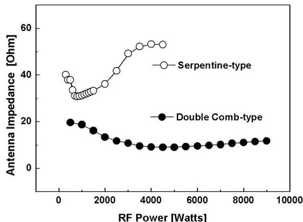
Fig. 4. Impedance measured as a function of rf power at 15 mTorr Ar by using an impedance analyzer for the serpentine-type antenna and double-comb-type antenna.
