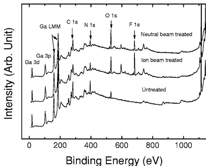
**Figure 3.** XPS wide-scan spectra for n-type GaN surfaces before and after treatments using both fluorine ion and neutral beams before BOE cleaning.
