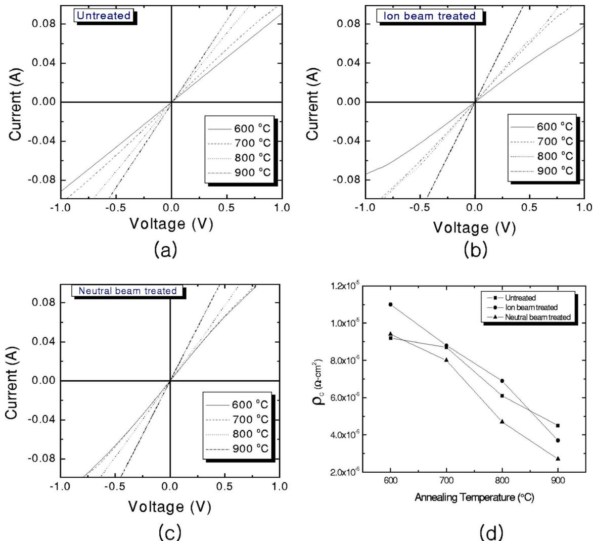
**Figure 2.** (Color online) Current-voltage characteristics of annealed Ti/Al/Au contacts on n-GaN treated by (c) fluorine neutral beam and (b) fluorine ion beam. (a) As a reference, the current-voltage characteristic of the contact fabricated on the untreated n-GaN was included. The variations in the specific contact resistivity and sheet resistance for all samples are also shown in (d).
