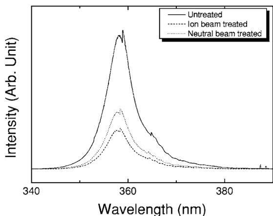
**Figure 5.** Room-temperature PL spectra of n-type GaN before and after treatments using both fluorine ion and neutral beams.
