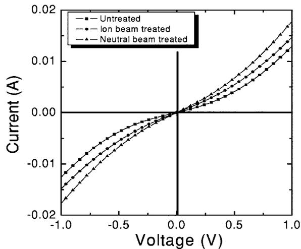
**Figure 1.** Current-voltage characteristics of as-deposited Ti/Al/Au contacts on n-GaN treated by fluorine ion beam and neutral beam. As a reference, the current-voltage characteristic of the contact fabricated on the untreated n-GaN was included.
