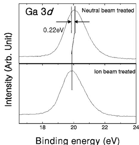
**Figure 4.** XPS narrow scan spectra of Ga 3d core level for n-type GaN surfaces after treatments using both fluorine ion and neutral beams.
