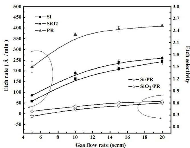
Fig. 3. Si, SiO<sub>2</sub>, and PR etch rates and etch selectivities of Si and SiO<sub>2</sub> to the PR as functions of the CF<sub>4</sub> flow rates to the source (rf power: 300 W; acceleration voltage: 400 V).
