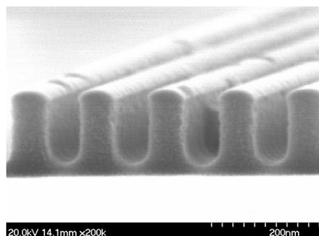
Fig. 5. SEM micrograph of the Si etch profile obtained by using a CF<sub>4</sub> neutral beam generated by the low-angle reflected neutral-beam source (rf power: 300 W; acceleration voltage: 400 V; CF<sub>4</sub> gas flow rate: 15 sccm).
