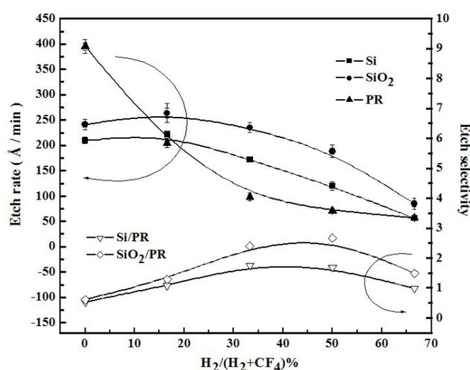
Fig. 4. Si, SiO<sub>2</sub>, and PR etch rates and etch selectivities of Si and SiO<sub>2</sub> to the PR as functions of the H<sub>2</sub> percentage in the CF<sub>4</sub>/H<sub>2</sub> mixture (rf power: 300 W; acceleration voltage: 400 V; total gas flow rate of the CF<sub>4</sub>/H<sub>2</sub> mixture: 15 sccm).
