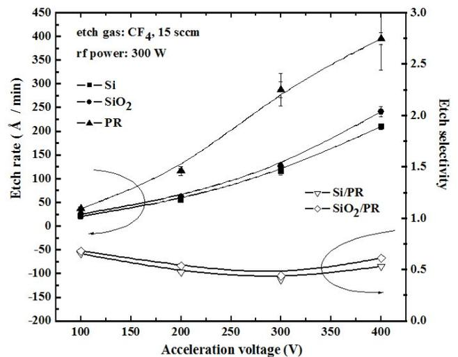
Fig. 2. Si,  $\text{SiO}_2$ , and PR etch rates and etch selectivities of Si and  $\text{SiO}_2$  to the PR as functions of the acceleration voltage of the source (rf power: 300 W;  $\text{CF}_4$  flow rate: 15 sccm).
