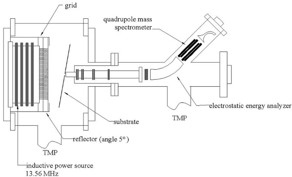
Fig. 1. Schematic diagram of the low-angle forward-reflected neutral-beam system used in the experiment.
