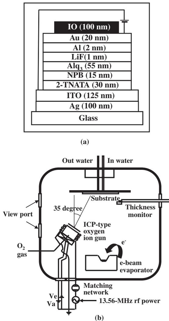
Fig. 1. (a) Schematic device configuration of the TEOLEDs fabricated. (b) The schematic diagram of the oxygen IBAD system used in the experiments.
