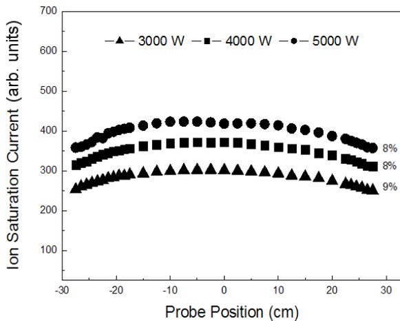
Fig. 6. Plasma uniformity measured 7.5 cm below each antenna as a function of the inductive power from 3000 to 5000 W for 15 mTorr of Ar. The ion saturation current measured using a Langmuir probe was used to estimation of plasma density.
