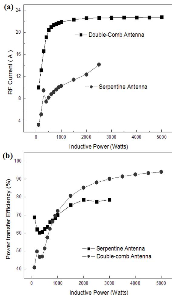
Fig. 5. (a) RF rms current of the antenna at the matching network position for the serpentine-type and the double-comb-type antennas as determined by using an impedance probe as a function of the inductive power from 100 to 5000 W at 15 mTorr of Ar. (b) Power transfer efficiency calculated for the two types of antennas as functions of the inductive power from 100 to 5000 W at 15 mTorr of Ar.
