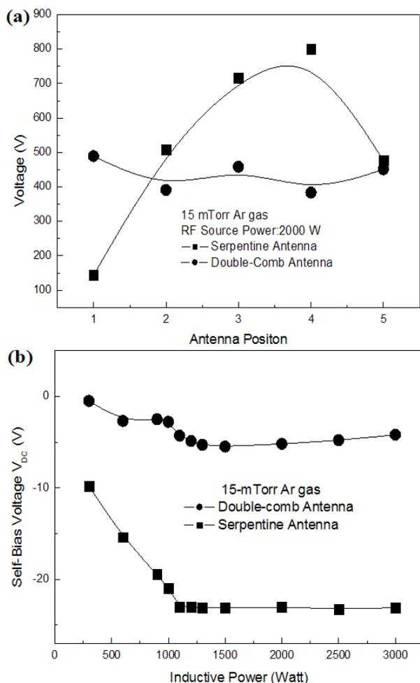
Fig. 4. (a) RMS voltage measured on the antenna line along the sidewall of the chamber for the double-comb-type antenna and the serpentine-type antenna for 15 mTorr of Ar and 2000 W of inductive power. (b) DC voltages induced on the dielectric surface covering the antenna line measured at a location close to the power input as a function of the inductive power at 15 mTorr of Ar for the two types of antennas.
