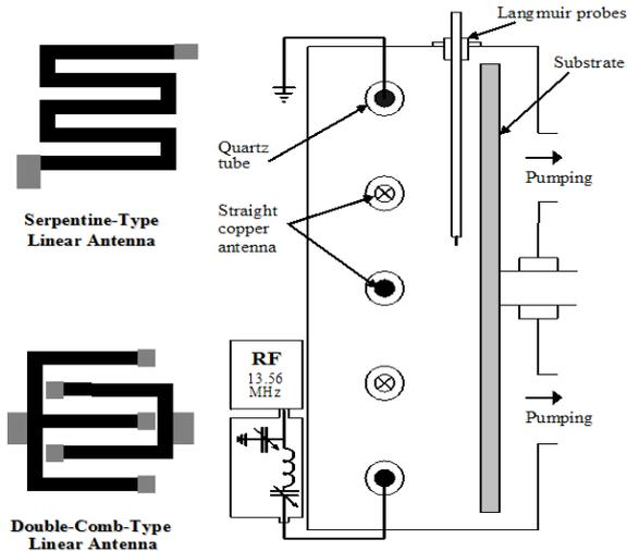
Fig. 1. Schematic diagram of the inductively coupled plasma system and the two types of internal linear antennas used in the experiment.
