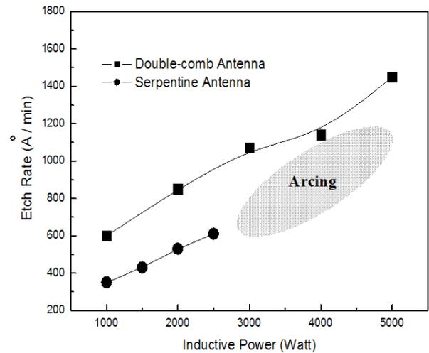
Fig. 3. Photoresist etch rates as a function of inductive power for 15 mTorr of  $\text{O}_2$  at a dc bias of -35 V for the two types of antennas.
