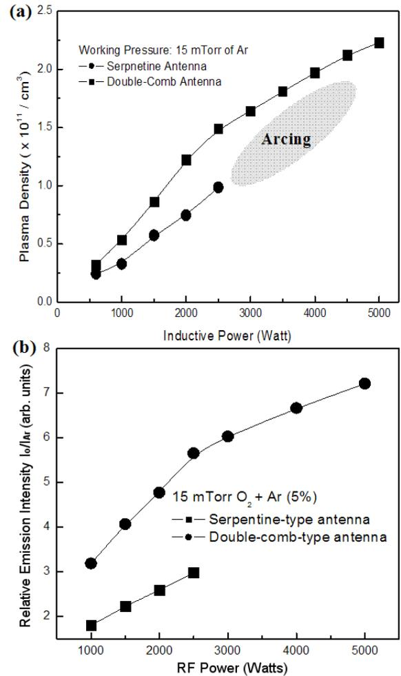
Fig. 2. (a) Ar ion density measured by using a Langmuir probe at 7.5 cm below each antenna as a function of the inductive power from 600 to 5000 W at 15 mTorr of Ar. (b) Relative oxygen atomic density estimated by using Ar actinometry for the serpentine-type antenna and the double comb-type antenna as functions of the inductive power from 1000 to 5000 W at 15 mTorr of O<sub>2</sub>.
