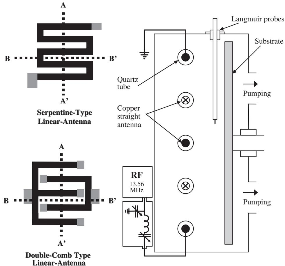
Fig. 1. Schematic diagram of inductively coupled plasma system and two types of internal linear antennas used in the experiment.
