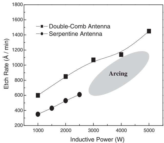
Fig. 3. Photoresist etch rates as a function of inductive power for 15 Torr O<sub>2</sub> and at -35 V of dc-bias voltage in two type antenna.
