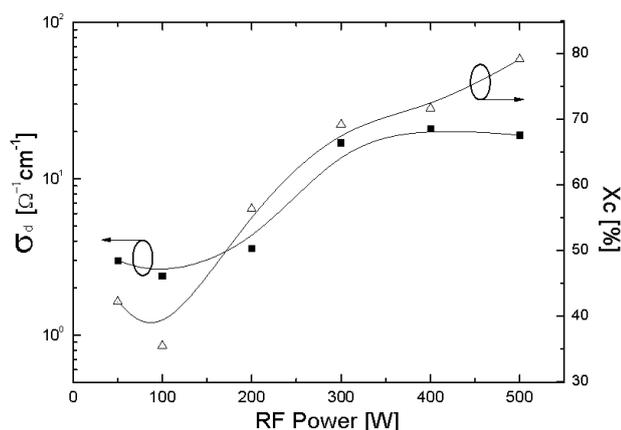
Fig. 7. The dark conductivity ( $\sigma_d$ ) of the silicon thin films deposited as a function of the rf power from 50 to 500 W.
