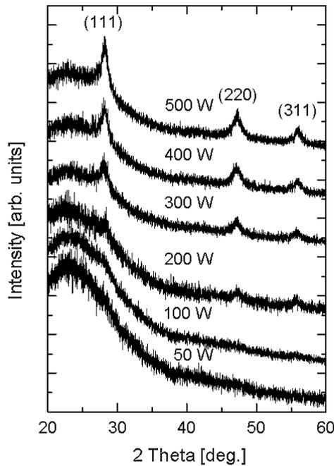
Fig. 5. XRD data of the deposited silicon thin films as a function of the rf power from 50 to 500 W.
