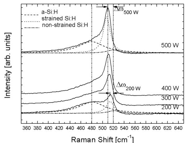
Fig. 2. Raman spectra of the hydrogenated silicon films deposited at various of rf source powers.
