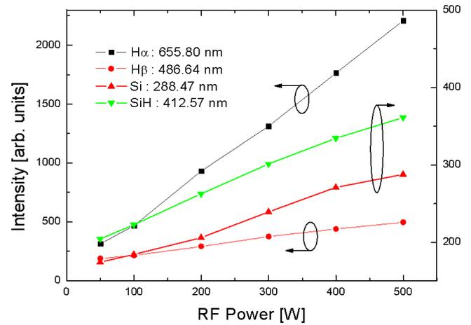
Fig. 4. Optical emission spectra of dissociated species, such as H, Si, and SiH, in the plasma as a function of the rf power from 50 to 500 W for a gas mixture composed of  $\text{SiH}_4$ ,  $\text{H}_2$ , and  $\text{PH}_3$ .
