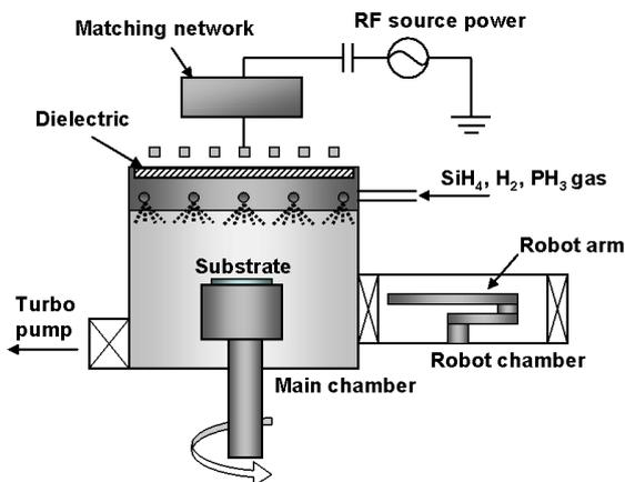
Fig. 1. Schematic diagram of the TCPCVD system used to deposit hydrogenated silicon films in this study.
