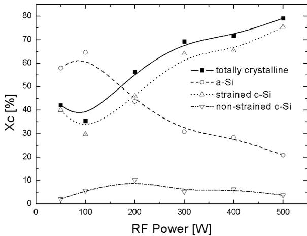
Fig. 3. Volume percentages ( $X_c$ ) of a-Si : H, strained c-Si : H, non-strained c-Si : H, and totally crystalline silicon of the deposited hydrogenated silicon thin films as a function of the rf power from 50 to 500 W.
