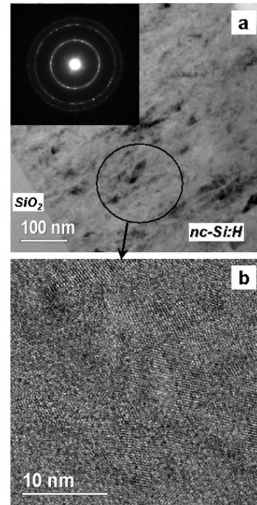
Fig. 6. TEM micrographs and diffraction patterns of the silicon thin film deposited at 500 W.
