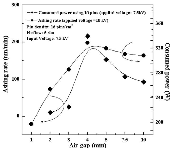
Fig. 5. Calculated consumed power measured as a function of the air gap for 16 pins/cm<sup>2</sup> at an applied voltage of 7.5 kV and a He flow rate of 5 slm. The photoresist ashing rate due to the residual oxygen gas in the He at an applied voltage of 10 kV is also shown.
