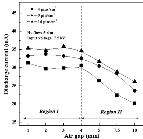
Fig. 4. Discharge current measured as a function of the air gap between the electrodes for various pin densities at an applied voltage of 7.5 kV and a He flow rate of 5 slm.
