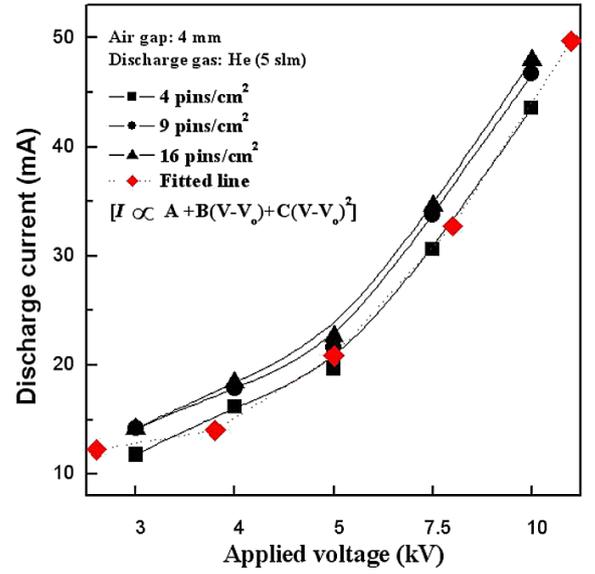
Fig. 2. Discharge current measured as a function of applied voltage for various pin densities of the power electrode at 5 slm of He. The air gap between the electrodes was 4 mm.
