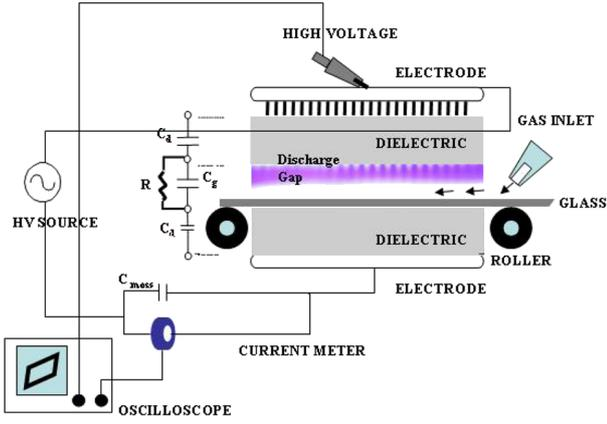
Fig. 1. The pin-to-plate DBD in-line system investigated to study the effects of the multi-pin density and the gap between the electrodes on the characteristics of atmospheric-pressure plasmas.
