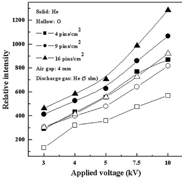
Fig. 3. Optical emission intensities from He metastable and oxygen atoms observed by OES as a function of the applied voltage for different pin densities of the power electrode. The air gap between the electrodes was 4 mm. The oxygen atomic emission intensities originated from the residual air during the atmospheric pressure operation.
