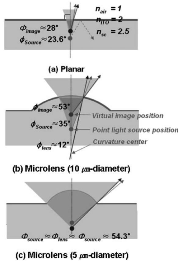
Fig. 3. Schematic diagram on the effect of micro-lens formed on the LLO GaN-based VLED devices on the increase of critical extraction angles for 5 μm and 10 μm micro-lens.
