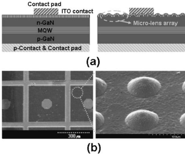
Fig. 1. (a) the schematic diagrams of the LLO GaN-based VLED devices with/without the micro-lens array formed in this study and (b) the scanning electron microscopic images of the 10 μm micro-lens array formed on the surface of n-GaN of the device.
