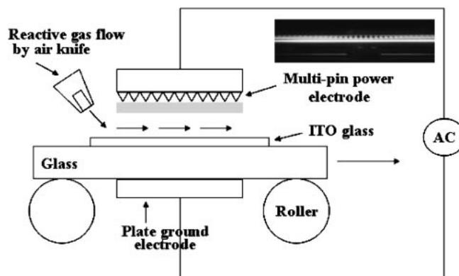
Fig. 1. Schematic diagram of the atmospheric pressure plasma equipment used for the surface treatment of ITO glass.
