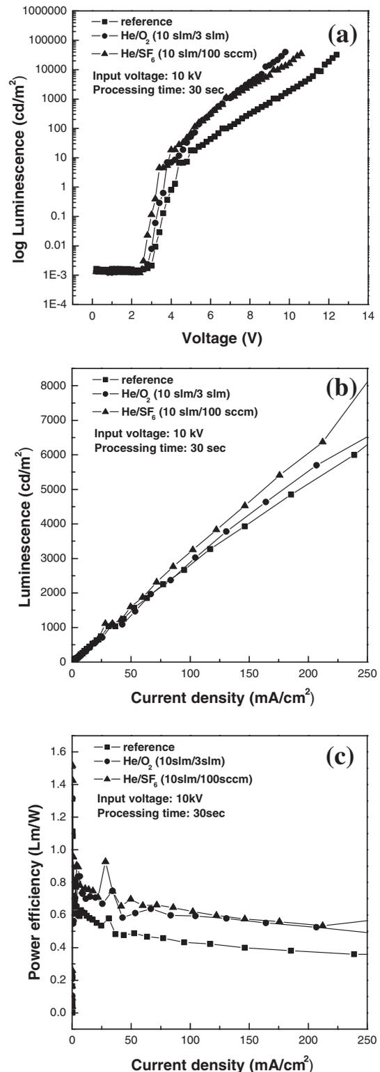
Fig. 2. Characteristics of the OLEDs fabricated on the ITO glass cleaned by the atmospheric pressure plasma using He(10 slm)/O<sub>2</sub>(3 slm) and He(10 slm)/SF<sub>6</sub>(100 sccm) gas mixtures. (a) luminescence-voltage, (b) luminescence-current density, and (c) power efficiency-current density. As a reference, the characteristics of the OLED device fabricated without plasma cleaning are included.
