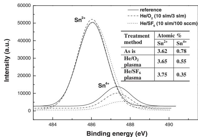
Fig. 3. Narrow scan XPS data of the deconvoluted Sn<sup>2+</sup> and Sn<sup>4+</sup> peaks from the Sn3d<sub>5/2</sub> peaks of the ITO surface treated with He(10 slm)/O<sub>2</sub>(3 slm) and He(10 slm)/SF<sub>6</sub>(100 sccm). The XPS data of the ITO surface not treated by the plasma is also included.
