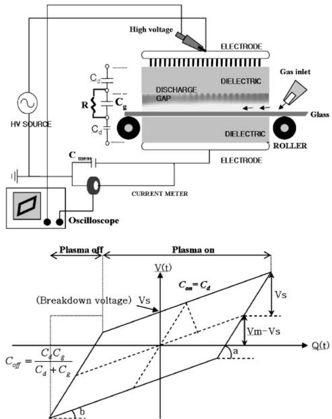
Fig. 1. (a) Schematic diagram of the atmospheric pressure plasma system (pin-to-plate type) and (b) the *Q*-*V* Lissarjou curve (*Q*-*V* oscillographic diagram) investigated in this study.
