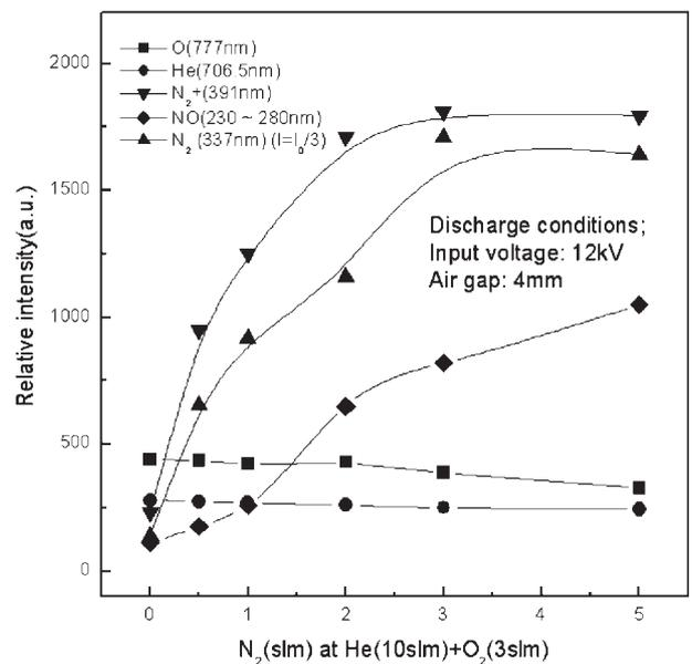
Fig. 3. Effect of N<sub>2</sub> flow rate in the He(10 slm)/O<sub>2</sub>(3 slm)/N<sub>2</sub>(0~5 slm) gas mixture on the relative optical emission intensities of He(706.5 nm), O(777 nm), N<sub>2</sub><sup>+</sup>(391 nm), N<sub>2</sub>(337 nm), and NO(230~280 nm; NO<sub>γ</sub> system) measured by OES.
