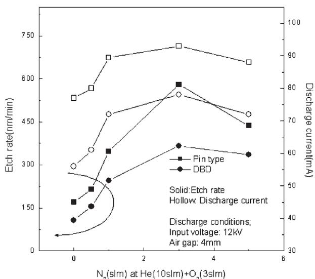
Fig. 4. Effects of  $N_2$  flow rate in the He(10 slm)/O<sub>2</sub>(3 slm)/N<sub>2</sub>(0~5 slm) gas mixture on the etch rates of photoresist and discharge rms currents at 12 kV of applied voltage. As a reference, the etch rates and discharge currents of a conventional DBD was included.
