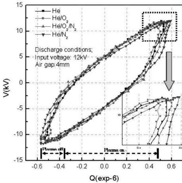
Fig. 2.  $Q$ - $V$  Lissajou curves of the discharges for the gas mixtures of He(10 slm), He(10 slm)/O<sub>2</sub>(3 slm), He(10 slm)/N<sub>2</sub>(3 slm), and He(10 slm)/O<sub>2</sub>(3 slm)/N<sub>2</sub>(3 slm) for the pin-to-plate type DBD having the electrode size of 100 mm × 1000 mm.
