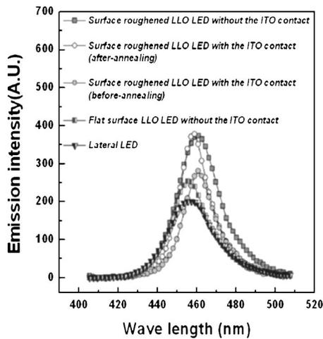
FIG. 4. Light emitting spectra of a conventional lateral GaN LED and the surface roughened LLO GaN VLEDs with a 100  $\mu\text{m}$  diameter Ti/Al contact and the nonpatterned ITO contact as the transparent current spreading layer.
