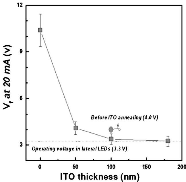
FIG. 2. Measured forward operating voltages of the LLO GaN VLEDs at an operating current of 20 mA as a function of the ITO layer thickness. When no ITO layer was deposited, a typical Ti/Al contact was used.
