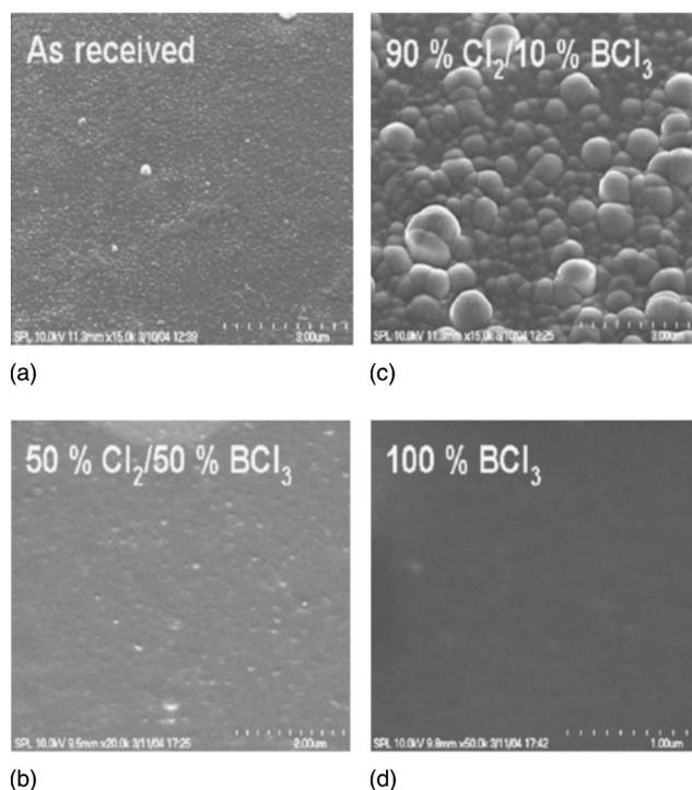
FIG. 1. Scanning electron micrographs of the LLO GaN device surface after etching using an ICP with various  $\text{BCl}_3/\text{Cl}_2$  mixtures: (a) as-received; (b) 10%  $\text{BCl}_3$ /90%  $\text{Cl}_2$ ; (c) 50%  $\text{BCl}_3$ /50%  $\text{Cl}_2$ ; and (d) 100%  $\text{BCl}_3$  at a gas flow rate of 100 sccm, a pressure of 10 mTorr, a rf power level of 1400 W, and a dc bias voltage of  $-150$  V.
