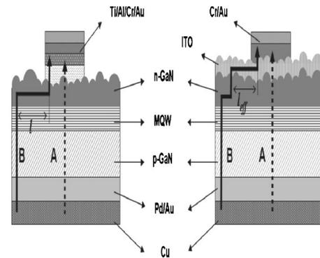
FIG. 3. Schematic diagram of the theoretical current paths of the LLO VLEDs with (a) a 100  $\mu\text{m}$  diameter Ti/Al contact and (b) with the nonpatterned ITO layer as the transparent current spreading layer.
