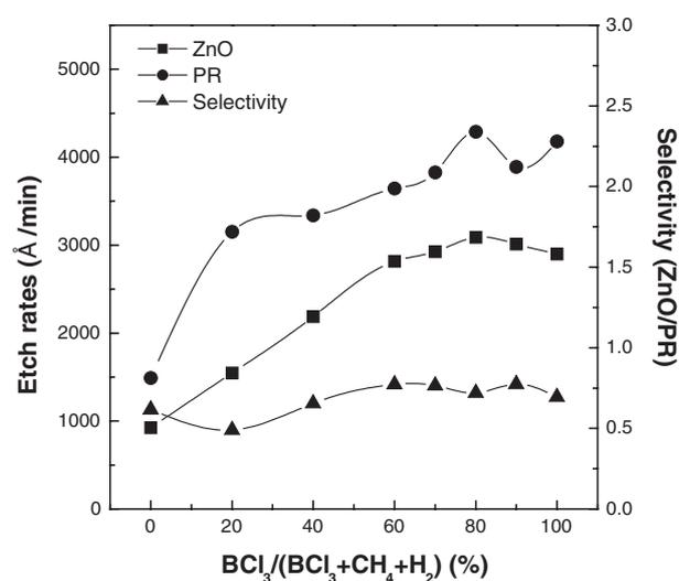
Fig. 1. Etch rate and selectivity over PR as a function of BCl<sub>3</sub> percentage in the BCl<sub>3</sub>/CH<sub>4</sub>/H<sub>2</sub> gas mixture (CH<sub>4</sub>/H<sub>2</sub> = 3:1) at rf power of 1200 W, working pressure of 5 mTorr, and bias voltage of −350 V.
