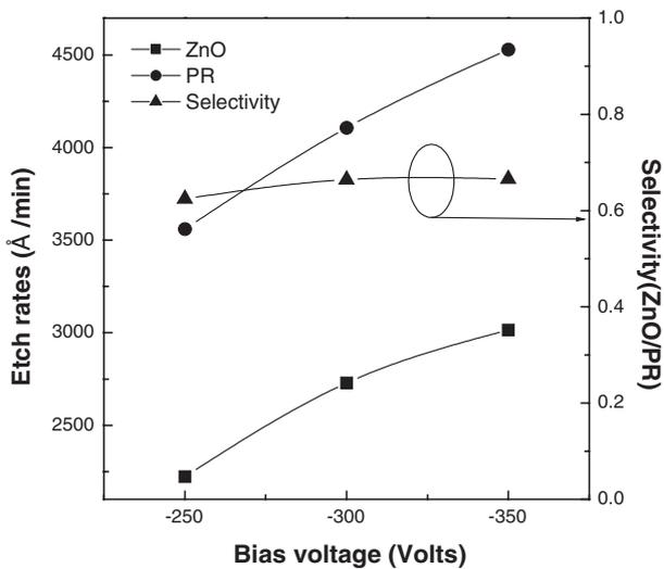
Fig. 2. Etch rate and selectivity over PR as a function of bias voltage for 80%  $\text{BCl}_3$  in the  $\text{BCl}_3/\text{CH}_4/\text{H}_2$  gas mixture ( $\text{CH}_3/\text{H}_2 = 3:1$ ), at rf power of 1200 W, working pressure of 5 mTorr, and substrate temperature of 20°C.
