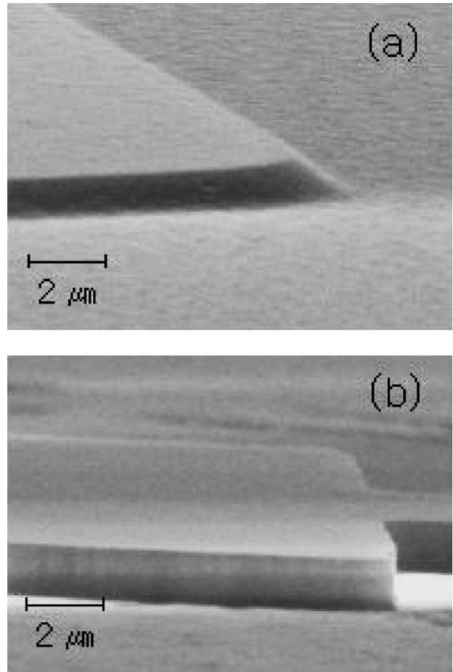
Fig. 3. SEM micrographs of AZO sidewall profiles etched with PR (a) and Cr masks (b) in 100%  $\text{BCl}_3$  plasma, at rf power of 900 W, working pressure of 5 mTorr, bias voltage of  $-350$  V, and substrate temperature of 20°C.
