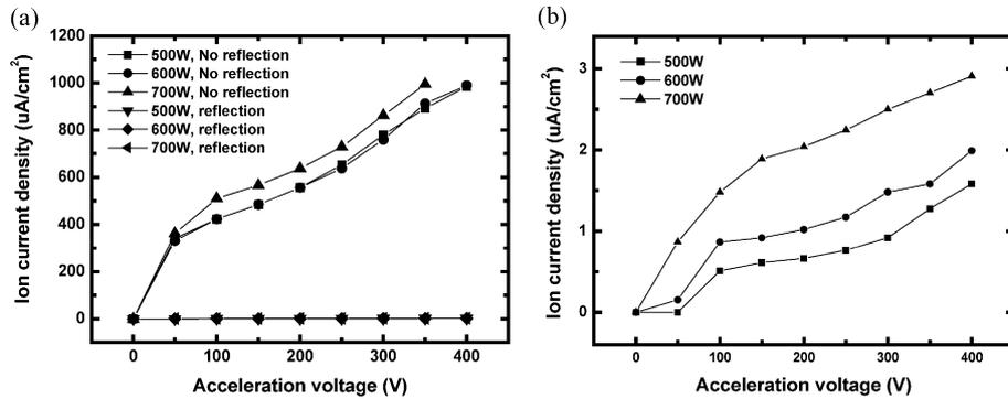
Fig. 1. Ion beam current density measured with a Faraday cup as a function of ion source acceleration voltage ( $V_a$ ) without reflector (a) and with reflector (b) for  $\text{SF}_6$  (rf power to ion gun: from 500 to 700 W; distance between the reflector and Faraday cup: 5 cm;  $\text{SF}_6$  flow rate: 7 sccm).
