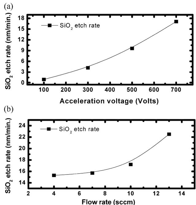
Fig. 2.  $\text{SiO}_2$  etch rate with the reflector as a function of acceleration voltage of the ion source for 7 sccm of  $\text{SF}_6$  gas flow rate (a) and as a function of gas flow rates of  $\text{SF}_6$  for 700 V of acceleration voltage (b) (rf power to ion gun: 500 W; distance between reflector and Faraday cup: 5 cm).
