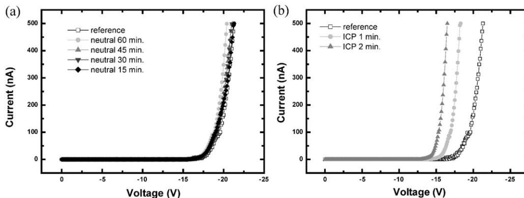
Fig. 3.  $I$ – $V$  characteristics of MOS devices exposed to oxygen neutral beam (a) or inductively coupled plasma (b) as a function of exposure time (oxygen neutral beam: 500 W of rf power, 0.7 mTorr (7 sccm) of oxygen, and 400 V of acceleration voltage; oxygen inductively coupled plasma: rf 500 W,  $-100$  V of bias voltage, and 5 mTorr of oxygen). To etch 1.2  $\mu\text{m}$  of photoresist, the oxygen inductively coupled plasma took 2 min while the oxygen neutral beam took 30 min.
