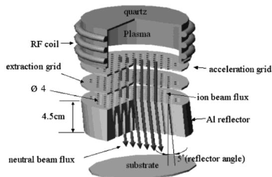
Fig. 1. Schematic diagram of the low-angle forward reflected neutral beam system used in the experiment.
