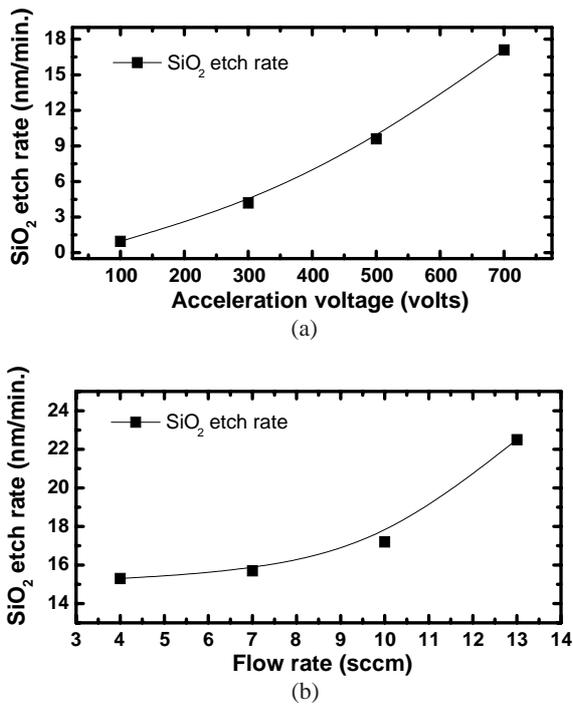
Fig. 2. SiO<sub>2</sub> etch rate with the reflector as a function of acceleration voltage of the ion source for 7 sccm of SF<sub>6</sub> gas flow rate (a) and as a function of gas flow rates of SF<sub>6</sub> for 700 V of acceleration voltage (b). (rf power to ion gun: 500 W, the distance between reflector and substrate: 5 cm.)
