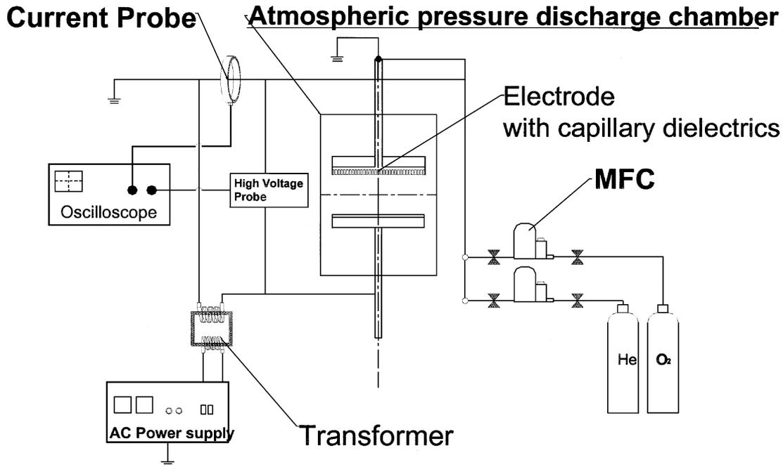
Fig. 1. Schematic diagram of dielectric barrier discharge system with capillary dielectrics used in the experiment.
