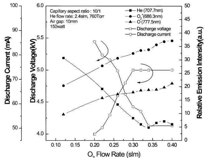
Fig. 5. The effect of  $O_2$  flow rate at 2.4 slm He flow rate on the discharge voltage, discharge current, and relative emission intensities of the discharges with capillary dielectrics.
