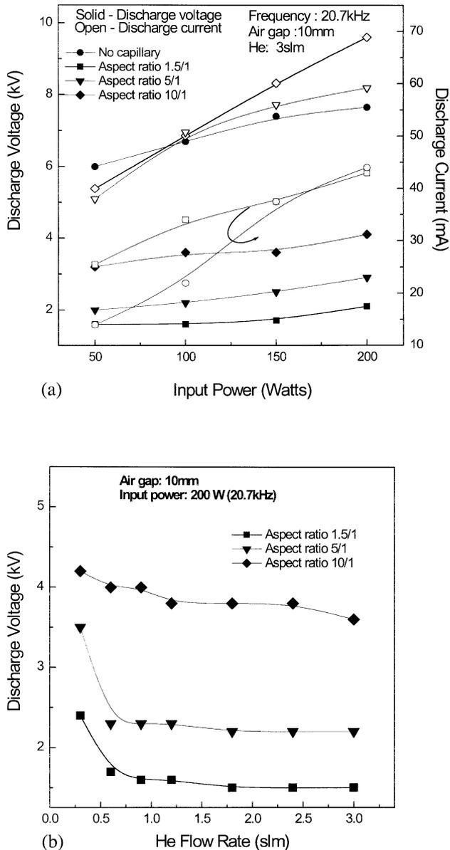
Fig. 2. The effects of input power (a) and He flow rate (b) on the discharge voltage and current for different hole aspect ratios of the electrodes with capillary dielectrics. Discharge voltage and current for the conventional dielectric barrier discharge was included in the figure to compare with the discharges with capillary dielectrics.
