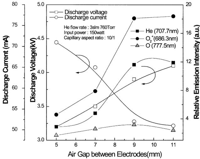
Fig. 4. The effects of air gap between the electrodes on the discharge voltage, discharge current, and relative emission intensities of the discharges with capillary dielectrics.
