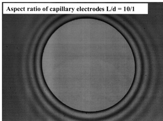
Fig. 6. Optical micrograph of photoresist clearing pattern in He (2.5 slm)/O<sub>2</sub> (0.2 slm), 20.7 kHz 200 W of input power, 10 mm of electrode gap, and the capillary aspect ratio of 10/1.
