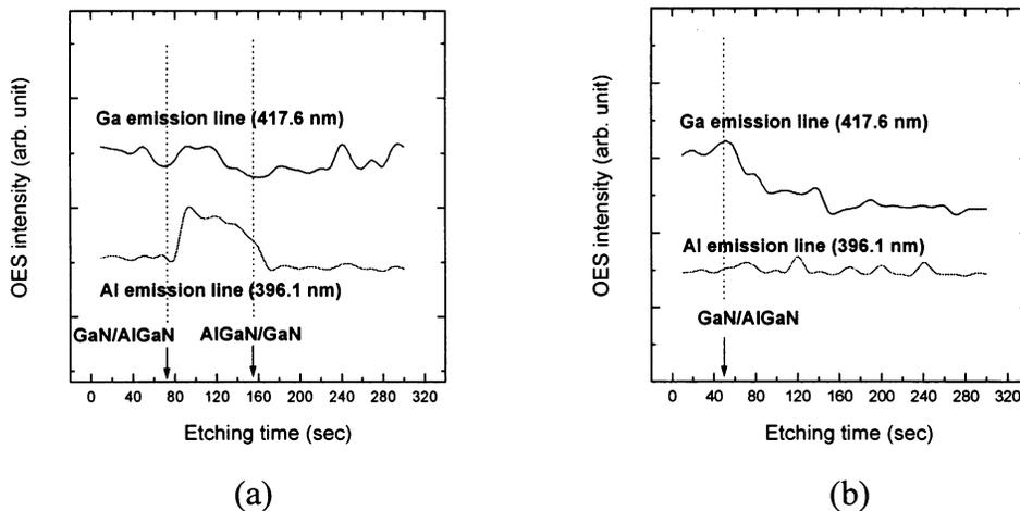
Fig. 1. (a) OES spectra during the etching of AlN, Al<sub>0.1</sub>Ga<sub>0.9</sub>N, and GaN and (b) the change of Ga and Al emission intensity during the etching of AlN (500nm)/Al<sub>0.1</sub>Ga<sub>0.9</sub>N (400 nm)/*n*-GaN (1500 nm)/*u*-GaN (500 nm) layer on the Al<sub>2</sub>O<sub>3</sub> substrate using etch II recipe shown in Table 1.
