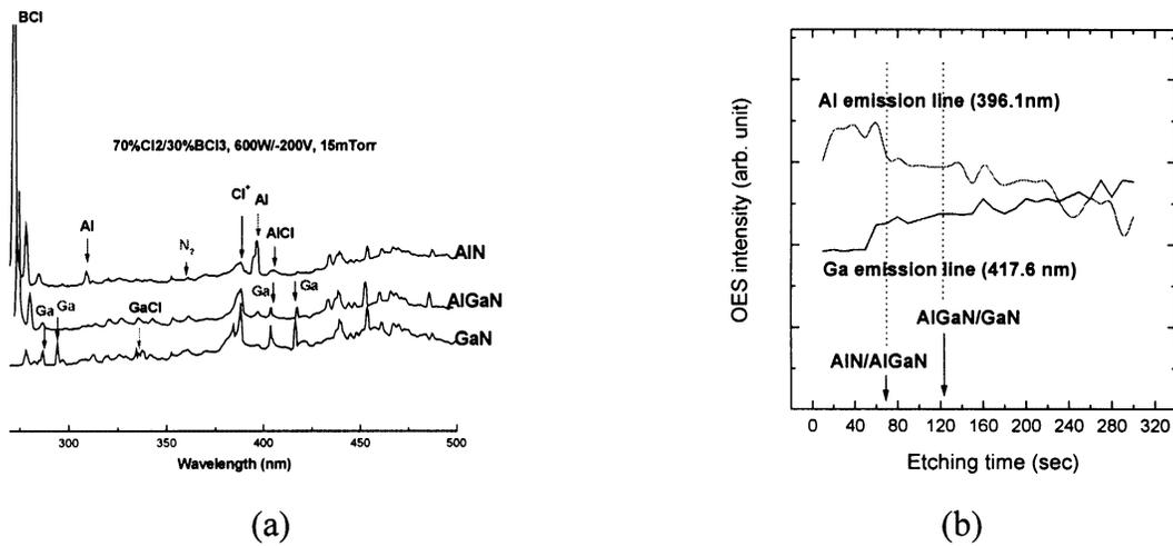
Fig. 2. The change of Ga and Al emission intensities during the etching of the GaN(700 nm)/Al<sub>0.17</sub>Ga<sub>0.83</sub>N/GaN(700 nm)/*n*-GaN(2000 nm) layer on the Al<sub>2</sub>O<sub>3</sub> substrate by (a) etch II recipe and (b) etch I recipe shown in Table 1.
