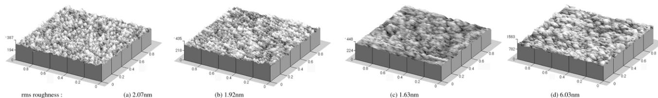
Fig. 3. AFM data showing the surfaces of ITO on polycarbonate as deposited: (a) and after the etching with; (b) 90% Ar/10% CH<sub>4</sub>; (c) 80% Ar/20% CH<sub>4</sub>; and (d) 70% Ar/30% CH<sub>4</sub>. Process conditions: 500 W of inductive power, -200 V of bias voltage, and 0.67 Pa of operation pressure.
