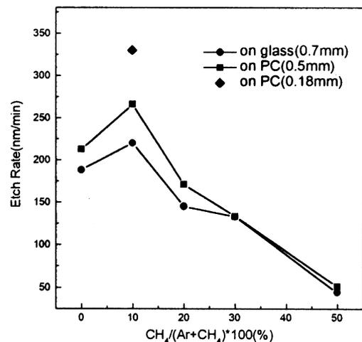
Fig. 2. Etch rates of ITO as a function Ar/CH<sub>4</sub> for both glass and plastic substrates in MICP. Process conditions: 500 W of inductive power, -200 V of bias voltage, and 0.67 Pa of operation pressure.
