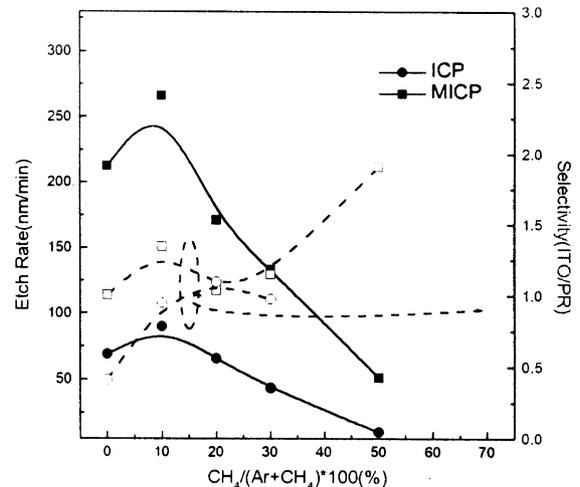
Fig. 1. Etch rates of ITO deposited on polycarbonate and their etch selectivities over photoresist as a function Ar/CH<sub>4</sub> for ICP and MICP. Process conditions: 500 W of inductive power, -200 V of bias voltage, and 0.67 Pa of operation pressure.
